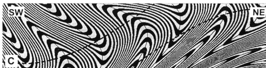
C) FINAL SITUATION PRODUCED BY SUPERIMPOSING LARGE SCALE DOME AND BASIN STRUCTURES (GIANBUL DOME) ON B
