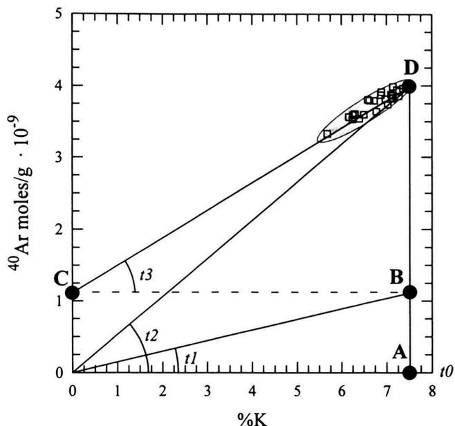
Fig. 7. %K -  $^{40}\text{Ar}^*$  schematic diagram showing a model for extraneous argon accumulation in chlorite during their formation. Legend: (A) biotite at formation time  $t_0$ , (B) biotite at time  $t_1$ , (C) chlorite formed at time  $t_1$  and (D) biotite at time  $t_2$ . See text for detailed explanation.
