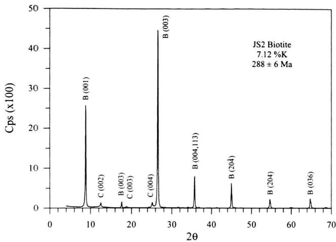
Fig. 3. X-ray spectra of biotite separate JS2. B and C represent the X-ray reflections for biotite and chlorite, respectively.
