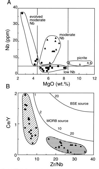
Fig. 4. (a) Nb. Mg diagram showing the division of the Migdhalitsa lavas into high Mg, low Nb, moderate Nb and evolved moderate Nb groups. (b) Ce/Y, Zr/Nb diagram showing the distribution of Migdhalitsa basalts into two major groupings, low and moderate Nb consistent with low and high degrees of partial melting.
