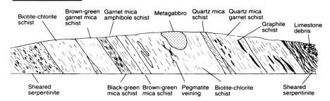
Fig. 10. Cross section of the metamorphic thrust sheet on the Lighourion/ Palea Epidavros road. Note the large competent block of gabbro in the center of the cutting.
