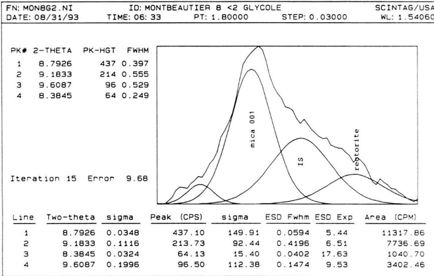
Fig. 12. X-ray diffraction pattern presenting reflections of mica 001, mixed-layers (IS) and rectorite near 10°2θ CuKα<sub>1</sub>.
