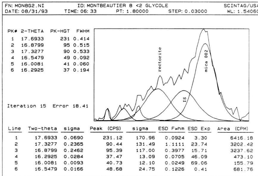
Fig. 13. X-ray diffraction pattern presenting reflections of mica 002, mixed-layers (IS) and rectorite between 16-17.7°2θ CuKα<sub>1</sub>.
