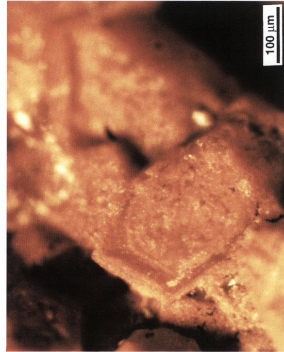
Fig. 4. Photomicrograph of a quartz crystal with several generations of growth rims. The light yellow parts contain organic encrustations.
