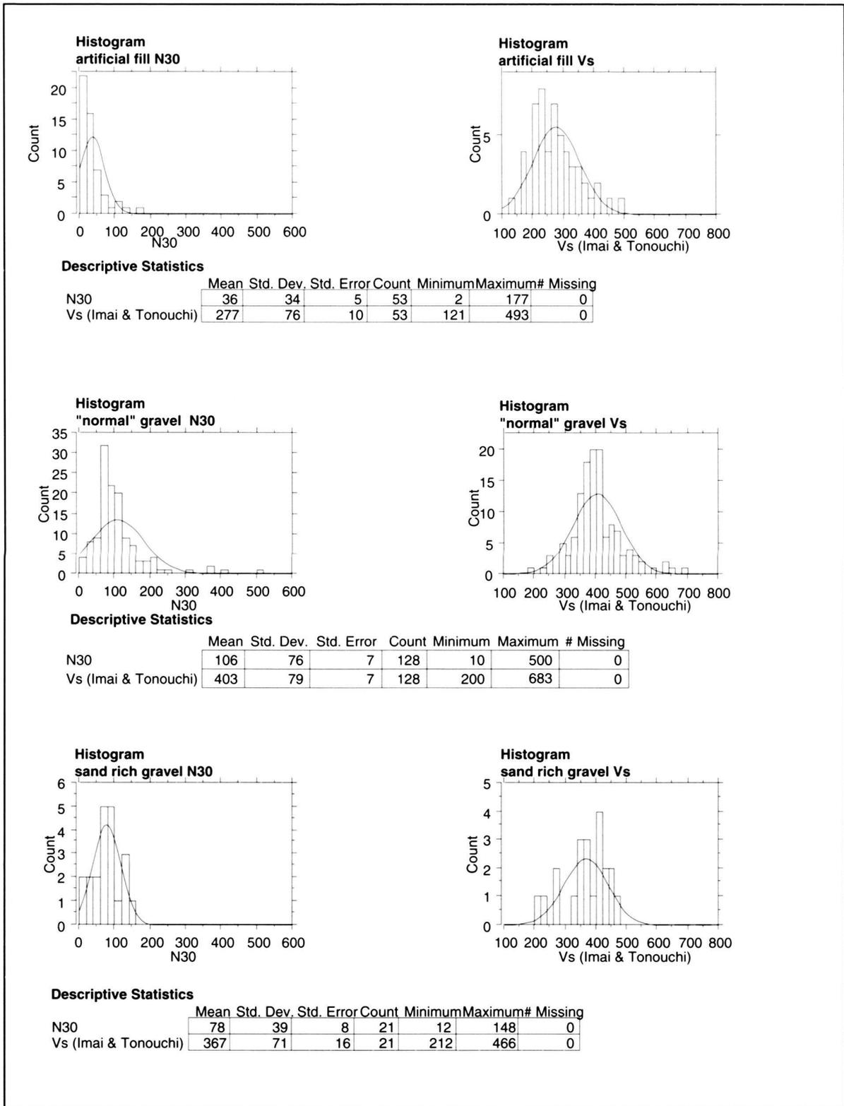
Fig. 4. Histograms for  $N_{30}$  of the different types of Quaternary gravels. The corresponding S-wave velocities are calculated after the empirical relation given by Imai & Tonouchi (1982).
