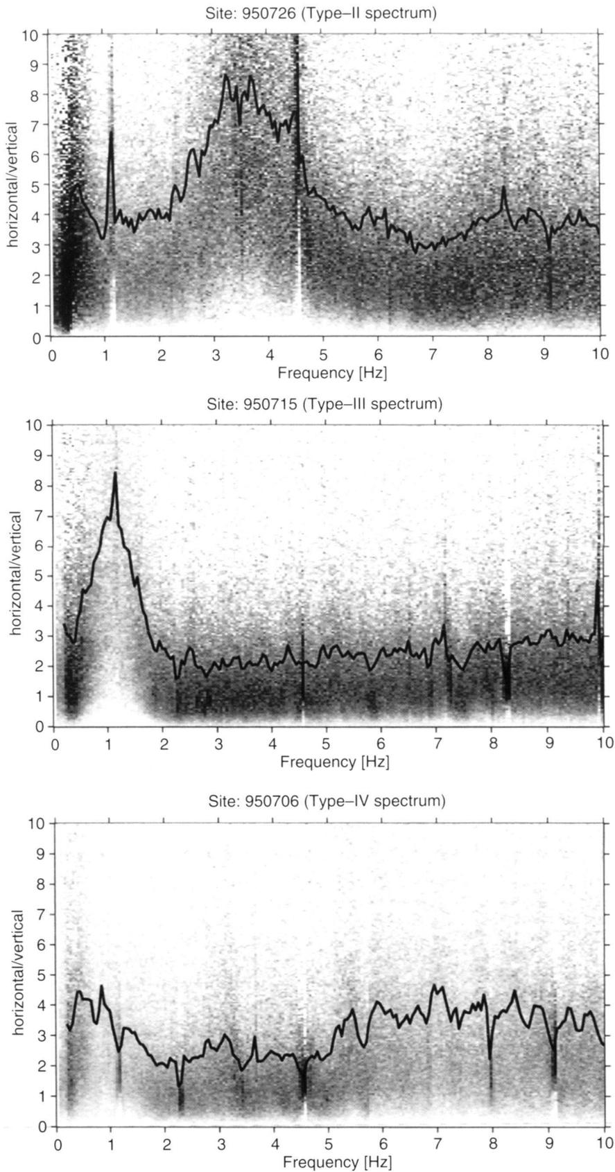
Fig. 5. Observed ambient-noise polarization spectra of types II, III and IV. Polarization is defined as the ratio between the Fourier spectrum of the horizontal components and the one of the vertical component. The solid lines correspond to the average polarization for all noise samples.
