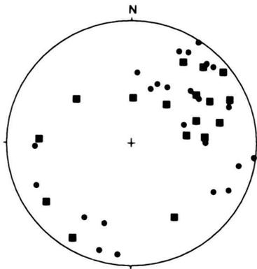
Fig. 3. Poles to 41 minor fault planes measured in some outcrops of the Malare unit (*Ma1* and *Ma3* formations). Dots and squares distinguish planes on which the pitch of striations is respectively high and low.
