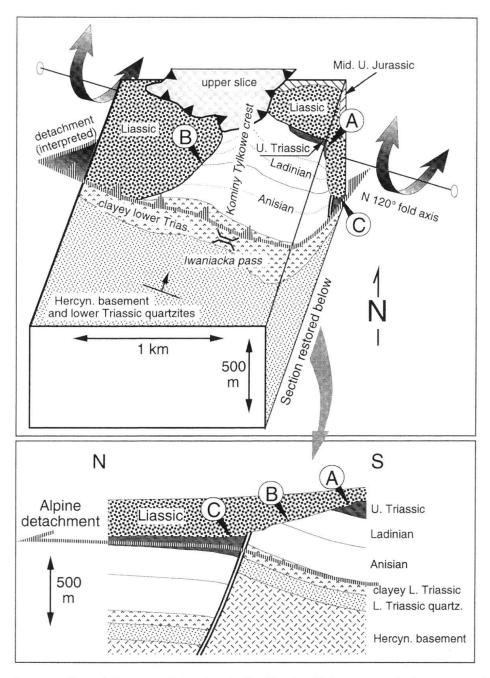
Fig. 6. top: interpretation of the present structure in the Kominy Tylkowe area; bottom: restoration of this structure. We propose that the rapid westward pinching-out of the Middle Triassic series (white) is a combined result of Latest Triassic-Early Liassic erosion and of Alpine detachment. A, B and C indicate outcrops located on Fig. 5.
