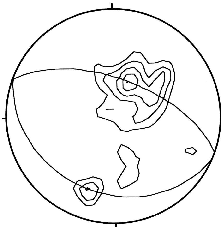
Fig. 4. Plot of the overall restored foliation poles (m. 200). Two main systems are defined at 90–100° to each other, the main system dipping 20–30° towards SW (equal area projection, lower hemisphere contours at 2–3 etc. times unit).
