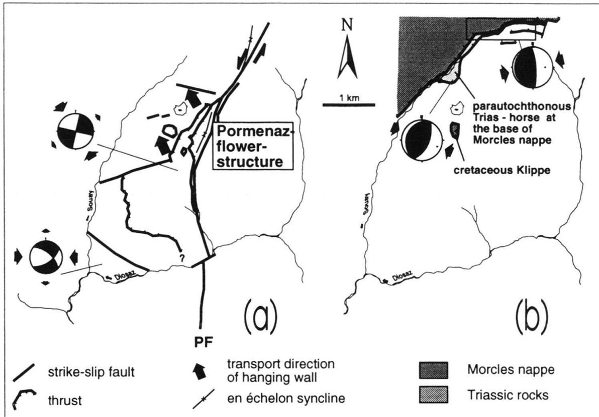
Fig. 4. Palaeostress analysis for a) pre-Oligocene transpression and b) Oligocene nappe emplacement. The different orientation of the nearly horizontal  $\sigma_1$ -axis gives evidence for anticlockwise rotation of the overall stress field during Tertiary deformation (see also Dobmeier 1994).
