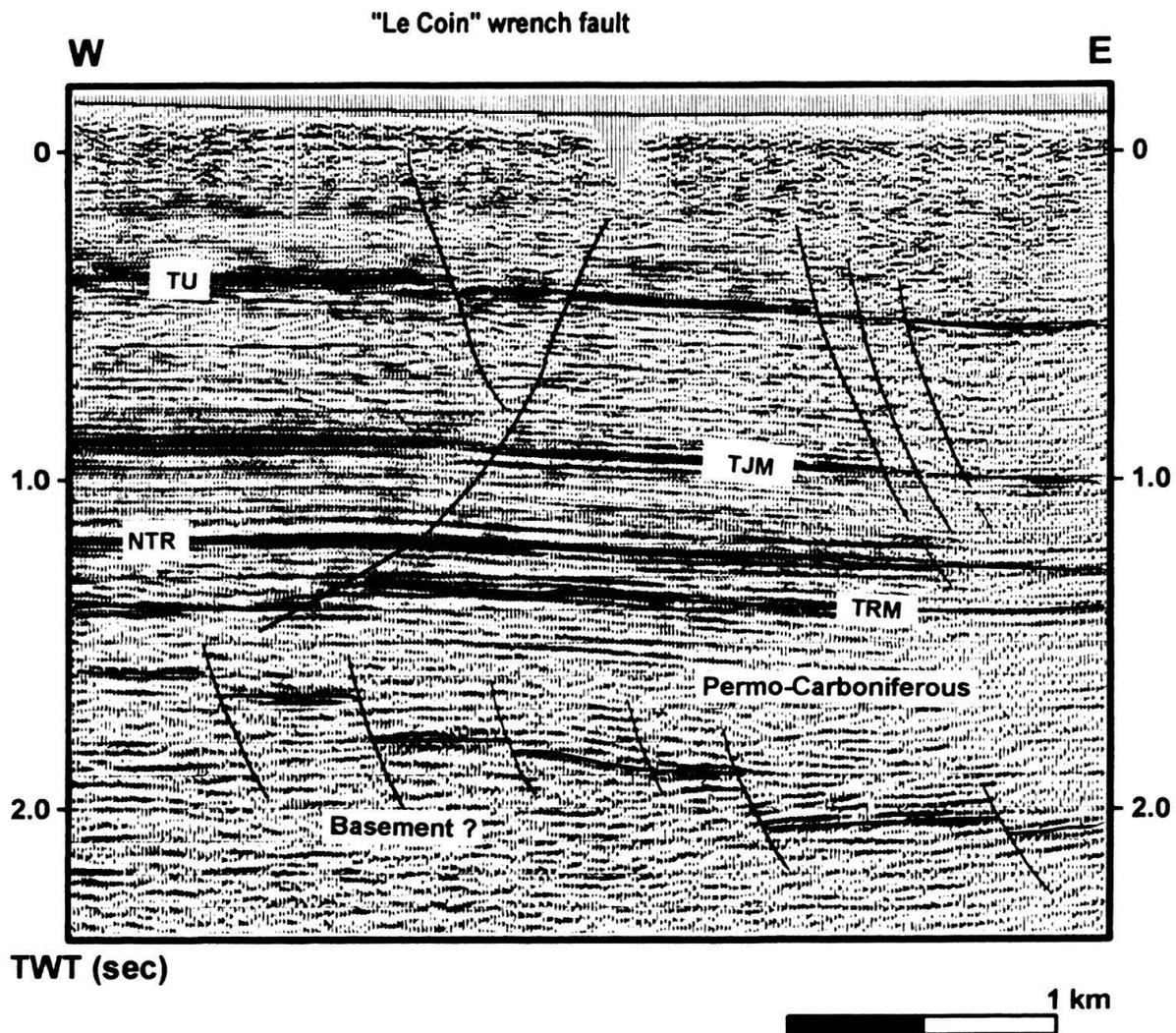
Fig. 9. Migrated seismic line in the Geneva Basin at the front of Mount Salève (see location on Fig. 7). This illustrates the subsurface continuation of “the Coin” wrench fault zone observed in Mount Salève: faulting in the Mesozoic-Cenozoic section overlies deep-seated Palaeozoic-basement faults. For abbreviations of seismic reflectors, see caption of figure 3.
