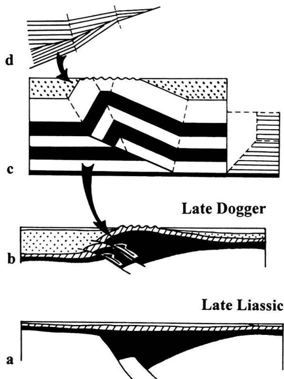
Fig. 10. Conceptual models related to the inversion of a half-graben (Bise-Tour d’Aï) redrawn with slight modifications from: a-b: Letouzey (1990); c: Mitra (1990), “fault propagation fold” in front of the Château d’Oche zone; d: Van Mount et al. (1990), progressive unconformity, onlaps and erosions as observed in the St Laurent cliff.
