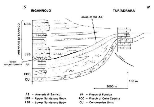
Fig. 9. Lithostratigraphic scheme of the proximal part of the Coniacian succession and interpretation of the relations with the Turonian units. Redrawn and modified after Bersezio et al. 1992.
