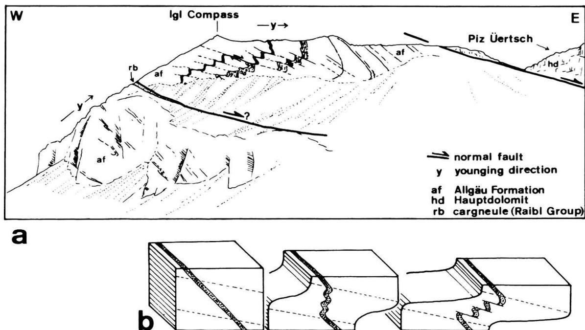
Fig. 11. D<sub>2</sub> structures at Igl Compass (Ela nappe north of Albula pass). (a) View of Igl Compass from south. Note regular arrangement of extensional shear zones in hinges of folds, suggesting that folds and shear zones originated from continuous process. (b) Model for continuous development of D<sub>2</sub> folds and extensional shear zones by top-east directed shearing deformation. Stippled layer is first shortened, then extended. After Froitzheim (1992).
