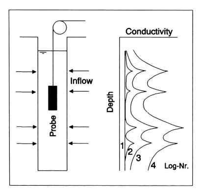
Fig. 1. Schematic representation of the fluid logging method
