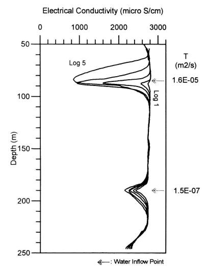
Fig. 3. Electrical conductivity logs measured at Burgdorf. Logging times are between 6 and 13 hours after flushing the borehole with brine (Ammann et al. 1993).
