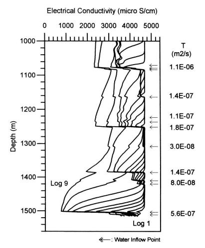
Fig. 2. Electrical conductivity logs measured in the Siblingen borehole. Logging times are between 1 and 37 hours after the start of pumping (Kelley et al. 1991).
