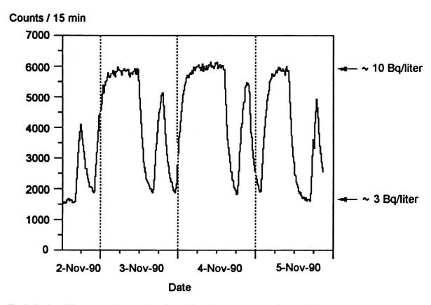
Fig. 3. Radon-222 concentration as a function of time for tap water at Fribourg, Switzerland.
