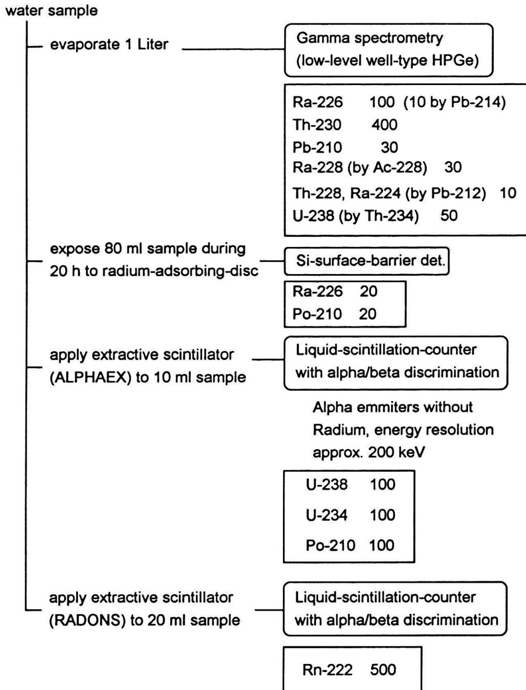
Fig. 2. Procedure for the analysis of natural radionuclides in drinking water. Numbers after nuclide names are typical detection limits in mBq/liter.
