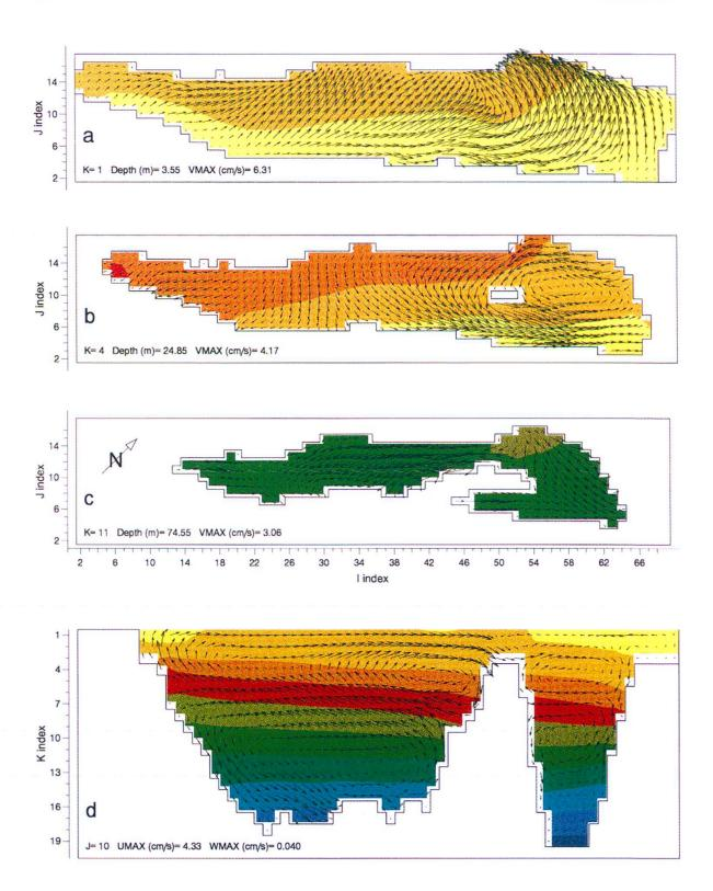
Fig. 5. Temperature and velocity fields (5a, b, c: horizontal sections, 5d: vertical section) six hours later the time corresponding to Figure 4. During this period, the wind has been turned off. Near the surface, the current is directed towards the NW coast and the water masses sink to feed a south-westward current in the deeper layers. In the vertical section, one notices the subdivision into two opposite rotating cells, epilimnetic and hypolimnetic.
