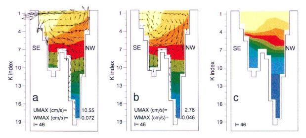
Fig. 6. Temperature and velocity fields (SE-NW transverse section) after a period of 12 hours of SW wind forcing with constant speed of 7.5 m/s (Fig. 6a) and six hours later, during which the wind has been turned off (Fig. 6b). Temperature field interpolated from measurements along the transverse section (Fig. 6c). The corresponding slice is indicated by the I value (see Fig. 2).
