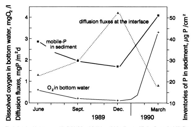
Fig. 6. Relationship between mobile-P (NAI-P and O-P) in surficial sediments, diffusion fluxes of soluble P at the interface and dissolved oxygen concentrations in bottom water in site Melide (data from LSA for dissolved oxygen content).
