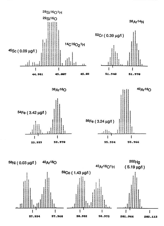
Fig. 3. Examples of molecular interferences observed in groundwater and polluted water samples using the HR-ICP-MS instrument.
