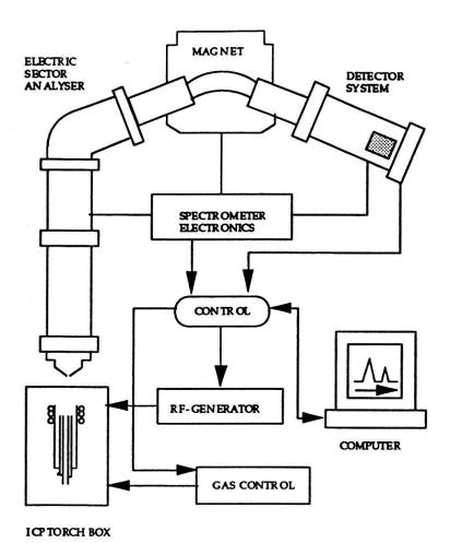
Fig. 1. Schematic diagram of the HR-ICP-MS instrument.
