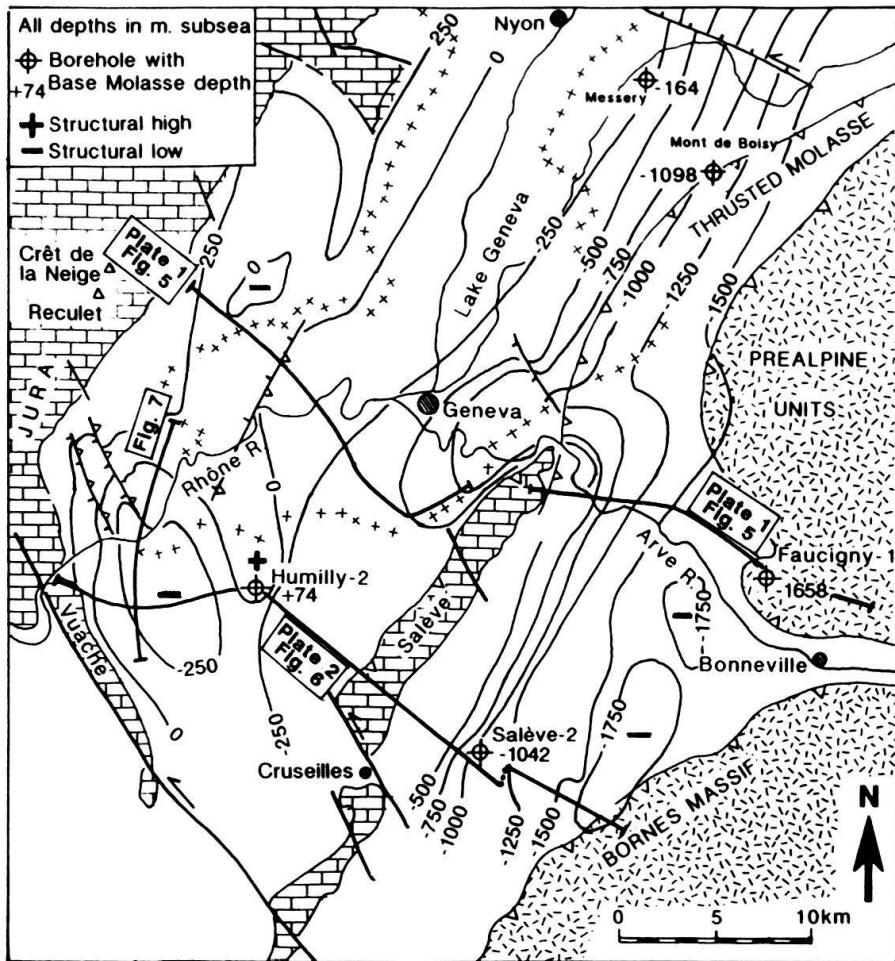
Fig. 2. Schematic Base Molasse depth map and location map in the greater Geneva area. This map connects with that of Figure 8.
