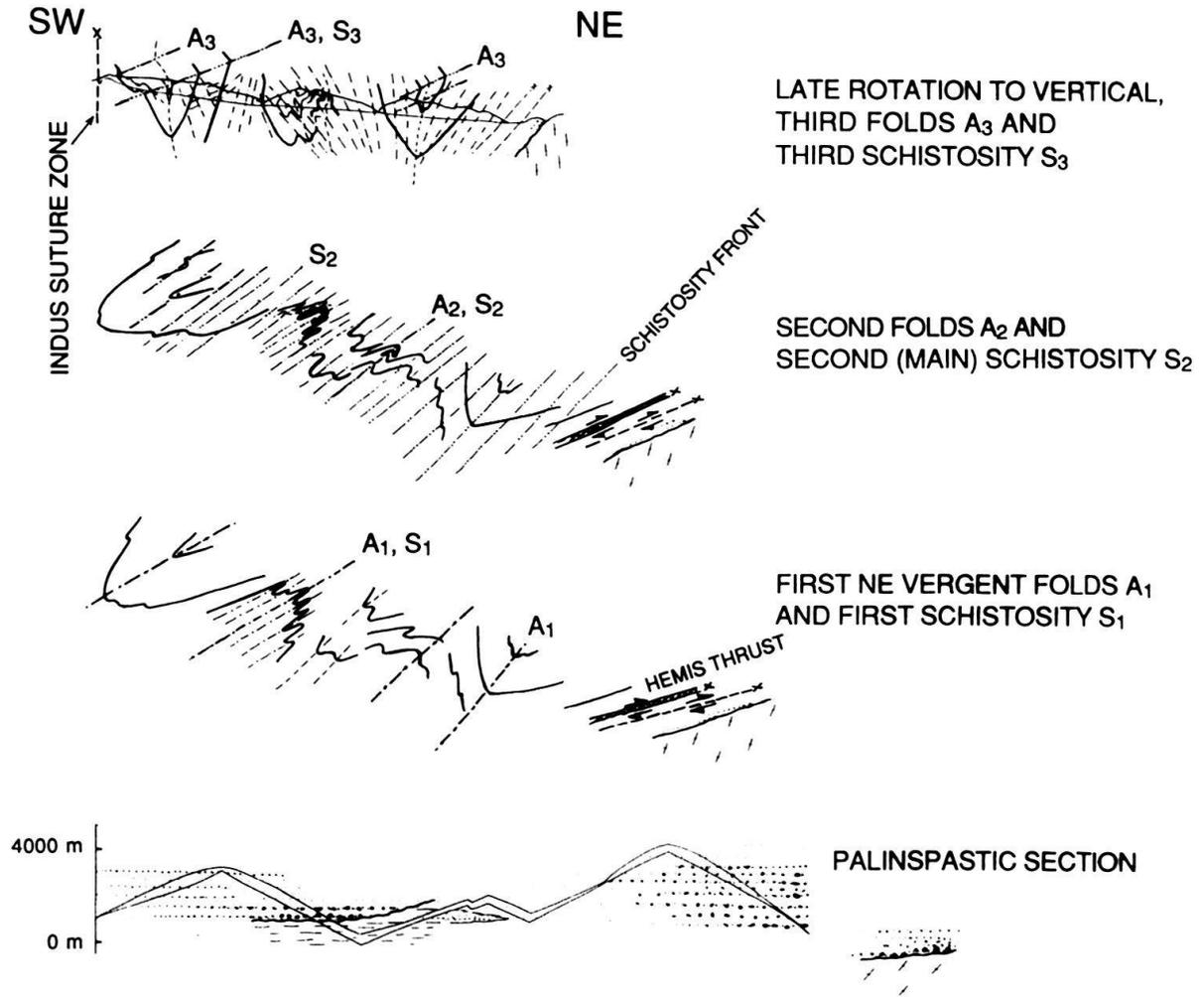
Fig. 7. Kinematic model for the NE vergent folding and thrusting of the Indus Molasse.  $A_1$ ,  $A_2$  and  $A_3$  = axial surfaces of  $F_1$ ,  $F_2$  and  $F_3$  folds respectively,  $S_1$ ,  $S_2$  and  $S_3$  = related schistosities.
