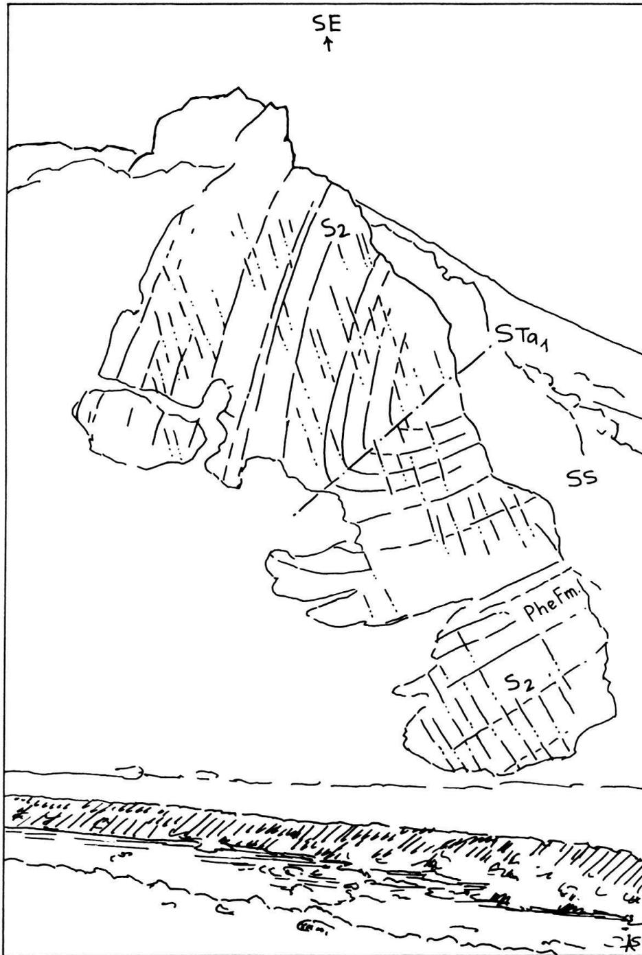
Fig. 29. NE vergent  $F_{Ta1}$  fold in the metamorphic sandstones of the lower Chandra Valley (Phe Fm. South of Batal), obliquely cut by the main schistosity  $S_2$ , related to the Baralacha La Thrust-Chandra Tal Flexure phase of deformation.
