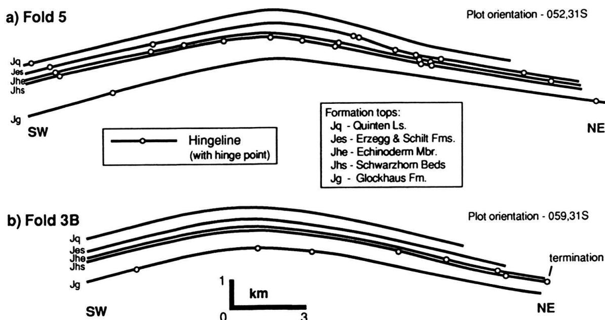
Fig. 10. Axial plane plots showing longitudinal geometries of: a) fold 5, and b) fold 3B. Hingelines are doubly-plunging away from fold culminations. The angle from horizontal is the pitch in the axial plane, not the true plunge (see text).
