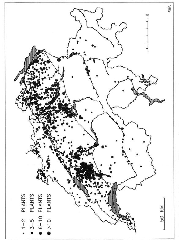
Fig. 5. Sites of installed vertical heat exchanger (VHE) systems. Installations of one commercial company only. Note the high VHE density in the Swiss Molasse Basin (highest worldwide). a: limit of the SMB.
