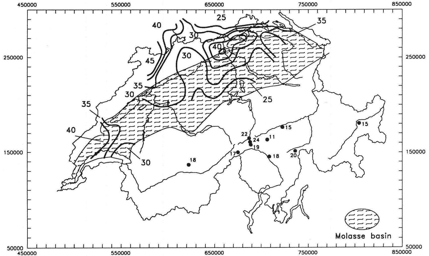
Fig. 1. Geothermal gradient data from Switzerland (in  $^{\circ}\text{C}/\text{km}$ ). The positive anomaly in the northeast coincides with the Permocarboneous trough (cf. Rybach et al. 1987).
