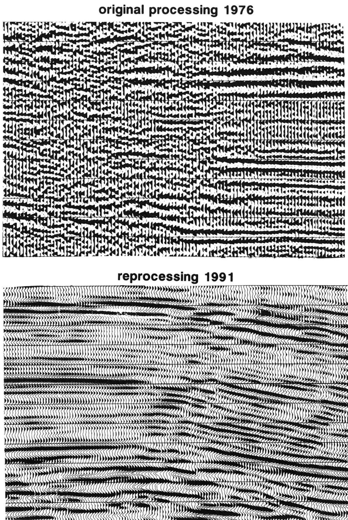
Fig. 13. Improvement by reprocessing of the 1976 seismic line (Swiss Molasse Basin)
