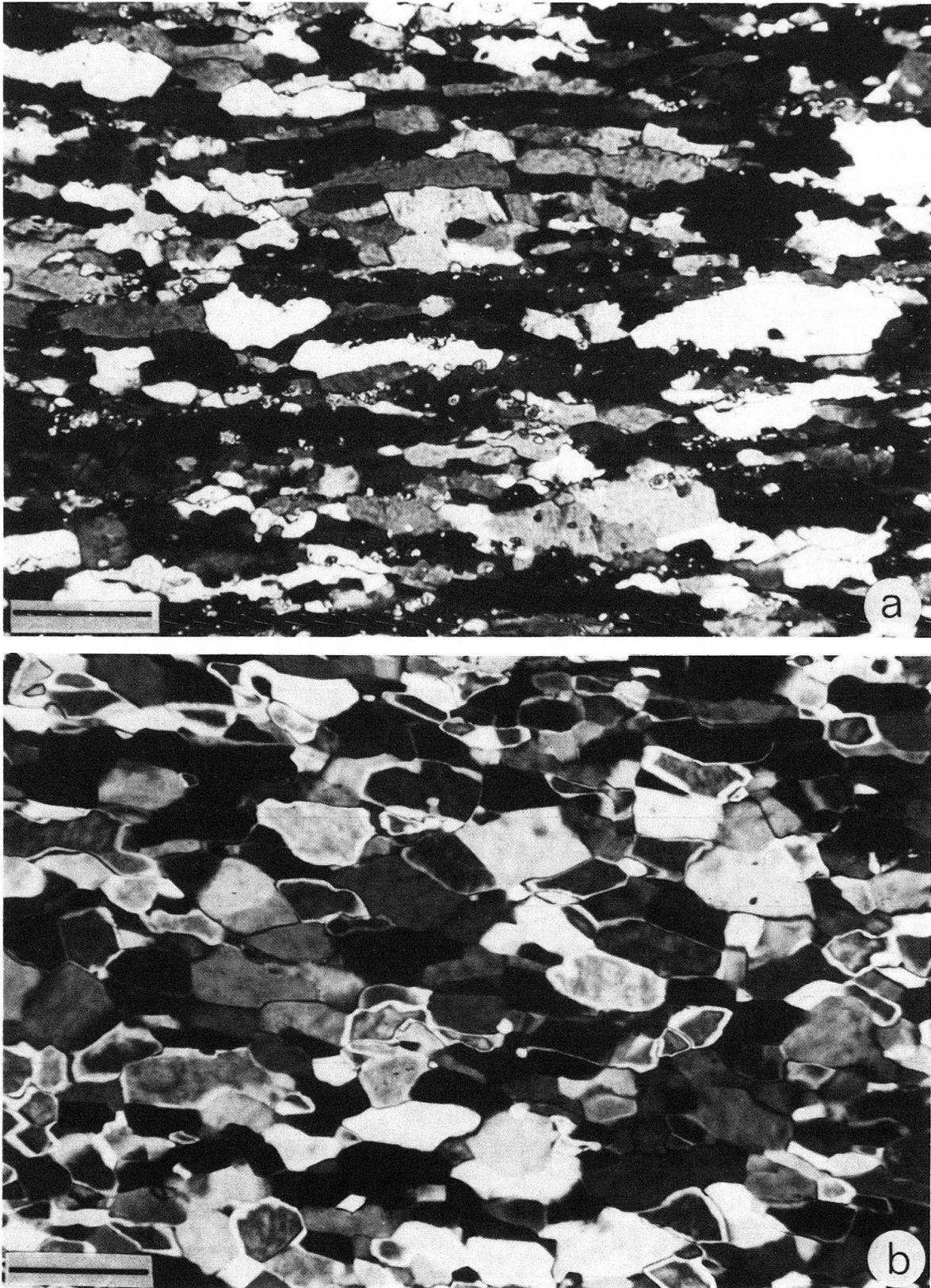
Fig. 6. Typical micrographs of two types of anhydrite mylonites (bar is 100  $\mu\text{m}$ ): a) from the Jura boundary thrust at Wisen, mainly deformed by crystal plasticity (regime 2); b) from the major sole thrust of Schafisheim, deformed by intracrystalline glide and diffusional or grain boundary sliding processes (regime 2/3).
