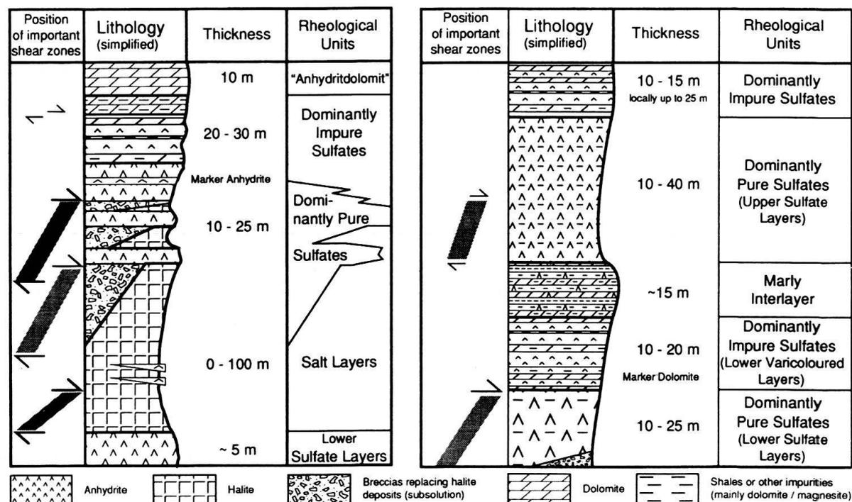
Fig. 1. Simplified stratigraphic columns of Middle Anhydritgruppe formation and Late Triassic Gipskeuper formation of the Eastern Jura and its hinterland showing the main rheological units and the location of the main decoupling horizons.
