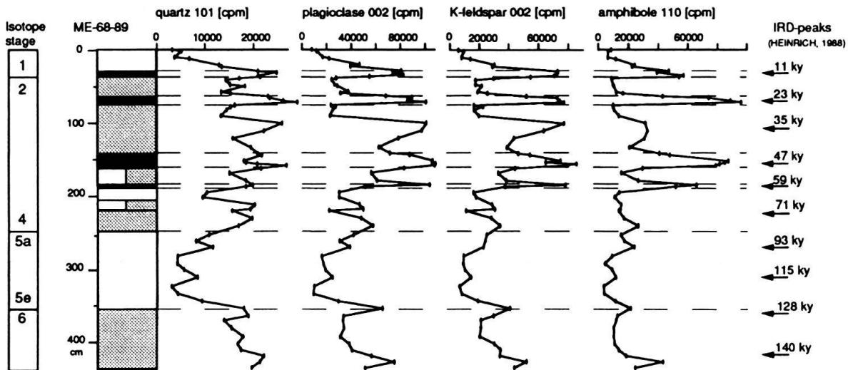
Fig. 5. Downcore distribution of quartz (101), plagioclase (002), K-feldspar (002) and amphibole (110) in the non-carbonate 2–16 µm fraction. Note the enrichment of amphibole in the cemented marl. Unit is cpm (counts per minute); for legend see Fig. 3.
