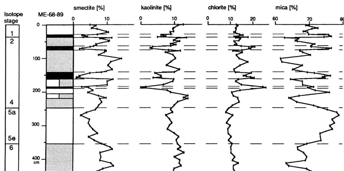
Fig. 4. Downcore distribution (core ME-68-89) of clay minerals (in relative %) in the non-carbonate < 2 µm fraction. Mineral percentages were calculated using the method of BISCAYE (1965). (for legend see Fig. 3).
