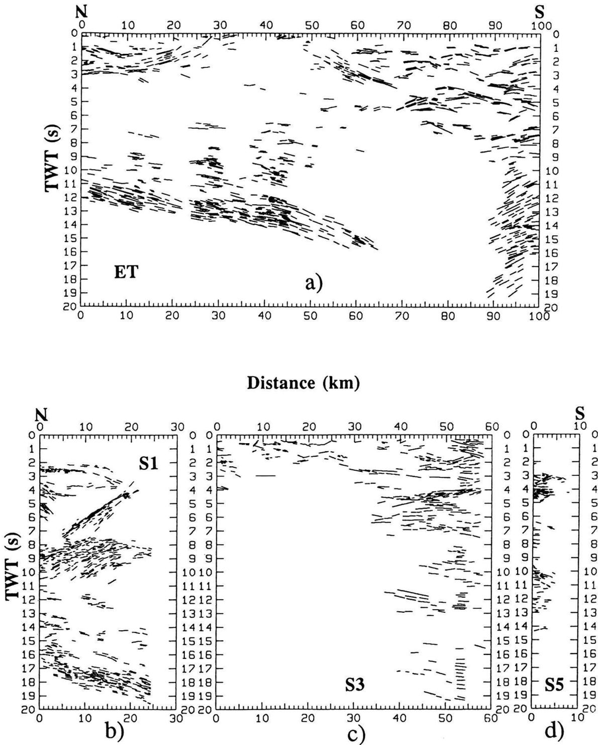
Fig. 8. Unmigrated digitized line drawings prepared from the NFP20 eastern and southern traverses. Horizontal (distance in km) and vertical (travel time in s) scales are 1:1 for an average crustal velocity of 6.0 km/s. For location see Figure 7.
