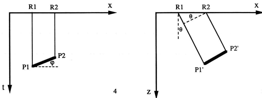
Fig. 4. Unmigrated line element defined by its end points  $P1$  and  $P2$  lying vertically below the corresponding coincident source/receiver locations  $R1$  and  $R2$ . Vertical axis is travel time, which is assumed to be scaled according to the “effective velocity” relevant for this line element.
