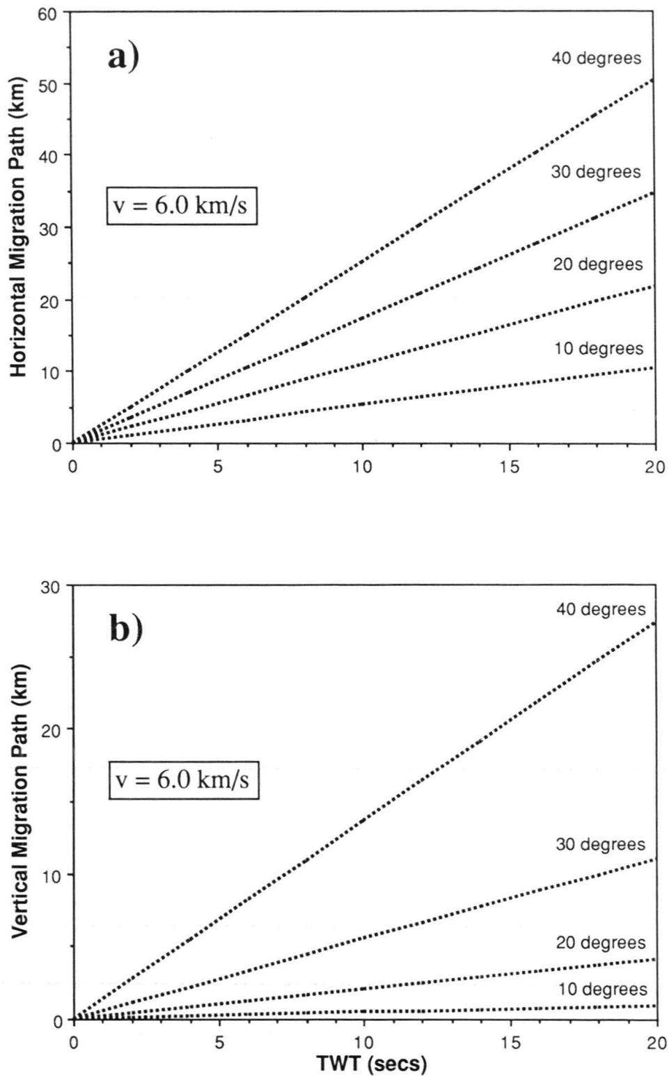
Fig. 2. Horizontal (a) and vertical (b) migration displacements as a function of apparent reflector dip and travel time. The velocity of the overburden is taken to be constant at 6.0 km/s, which is a representative average value for crustal studies.
