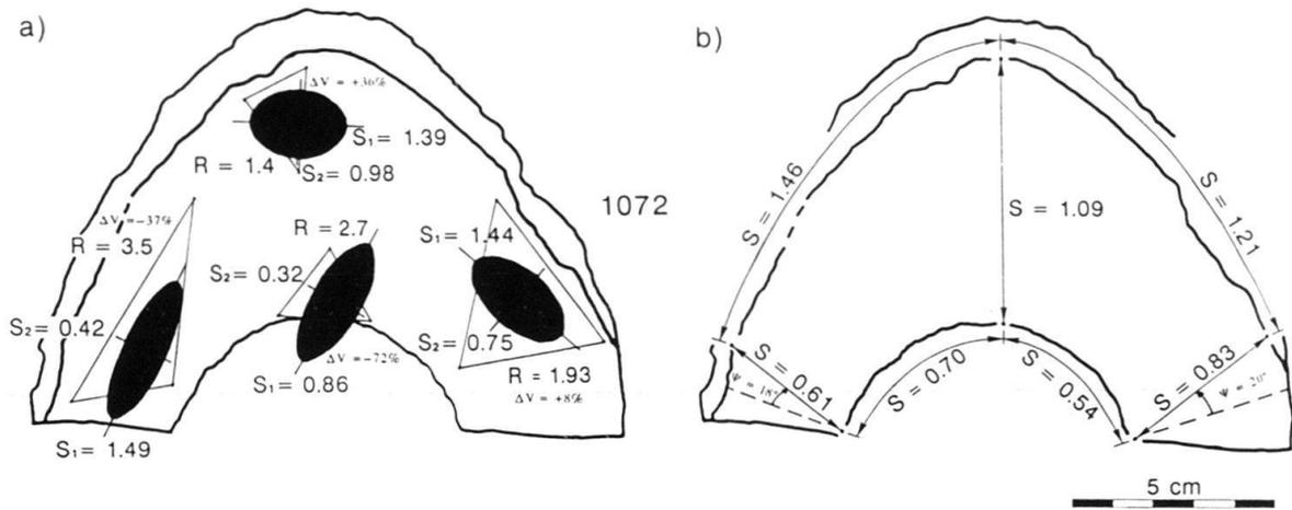
Fig. 8. Strain data for fold shown in Fig. 6a. a) Strain ellipses calculated from deformed and retrodeformed triangles.  $S_2$  and  $S_1$ : lengths of long and short axes of strain ellipse expressed as stretch ( $S = 1 + \Delta l/l_0$ ).  $\Delta V$ : volume change (positive for increase). b) Thickness variations and layer-parallel deformation expressed as stretch.  $\Psi$ : angular shear of line initially orthogonal to bedding.
