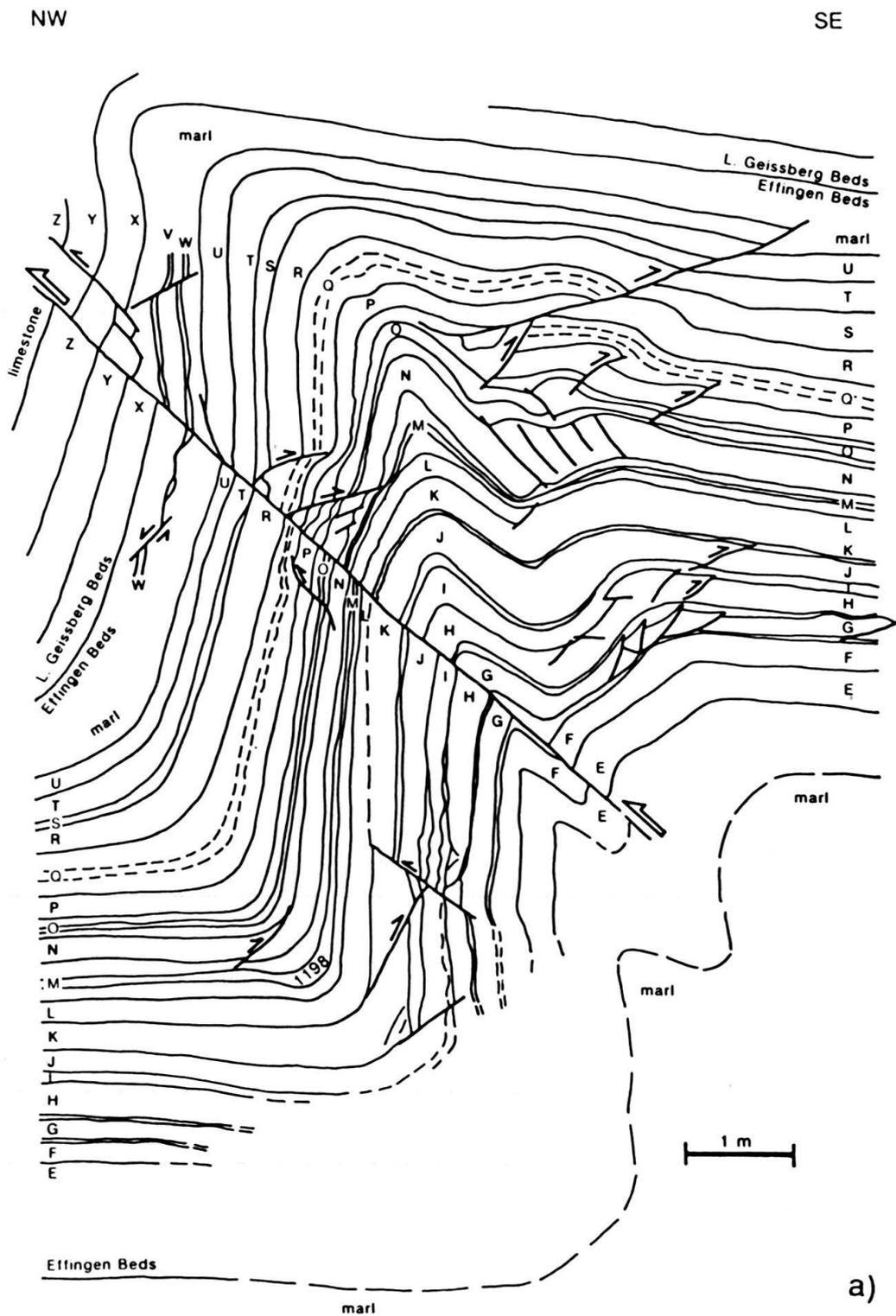
Fig. 3. Detailed cross sections from Fig. 2 (Les Prélaz) showing the complex interplay between folding and faulting. See text for discussion.
