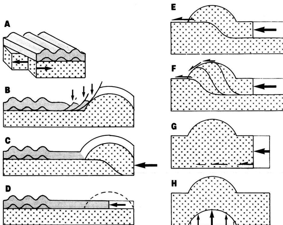
Fig. 2. Conceptual models of Jura- and/or Molasse-shortening and possible relationships with the external crystalline Aarmassif. A first series of sketches illustrates the four fundamentally different possibilities to explain shortening in the Jura (or Subalpine Molasse):
