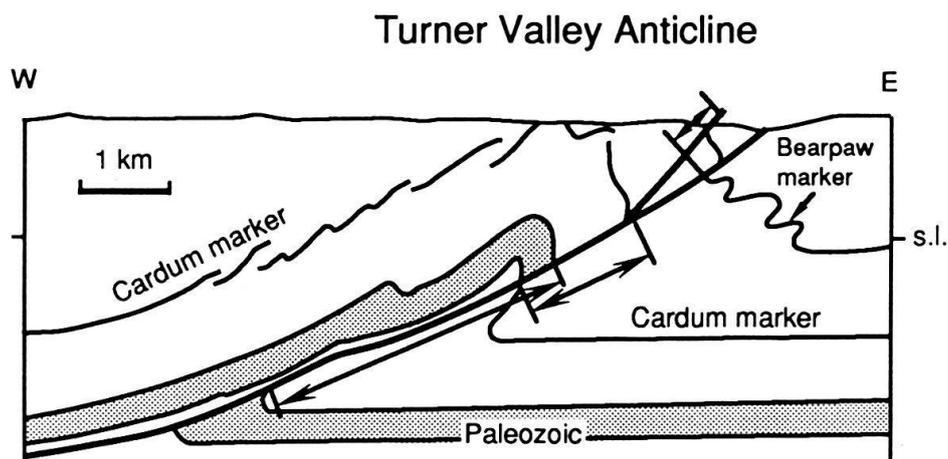
Fig. 4. Cross section of Turner Valley structure, Alberta discussed by DAHLSTROM (1970), as quoted in text.
