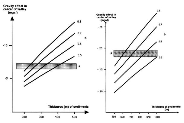
Fig. 7. (left) Gravity effect of prismatic bodies of various thickness and density for the sedimentary fill of the Valtellina at Sondrio (profile b2). The elevation of the Adda river is 288 m above sea level.
