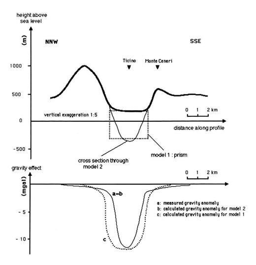
Fig. 4. Magadino Plain. Comparison between a prismatic model and a cross section through the 3D-model 2 based on seismic results (see text). While both model anomalies (b and c) are of equal amplitude (12 mgal) only the calculated anomaly (b) that belongs to the 3D-model fits the observed residual gravity anomaly (a). Model 2 has been used to calculate the density-depth function shown in Fig. 5.
