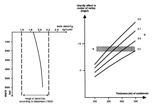
Fig. 5. (left) Density-depth function for sedimentary fill of Magadino Plain.
