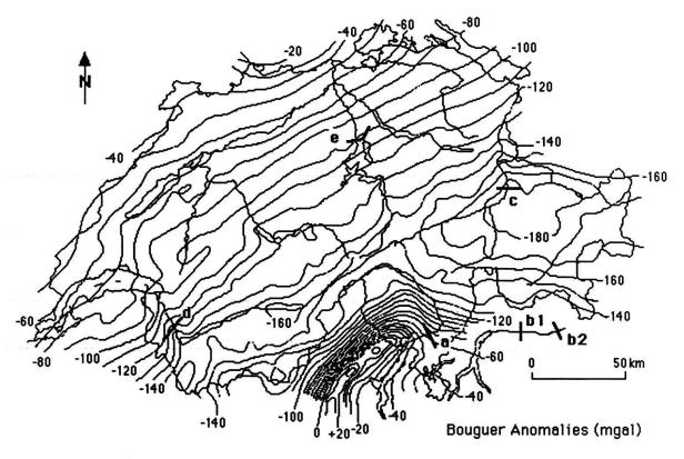
Fig. 1. Bouguer gravity map of Switzerland (KLINGELÉ & OLIVIER 1980; KISSLING 1980; SCHWENDENER 1984). Values are given in (mgal), where 1 mgal = 10<sup>-5</sup> ms<sup>-2</sup>. The locations of the Alpine valleys discussed in the text are marked with:
