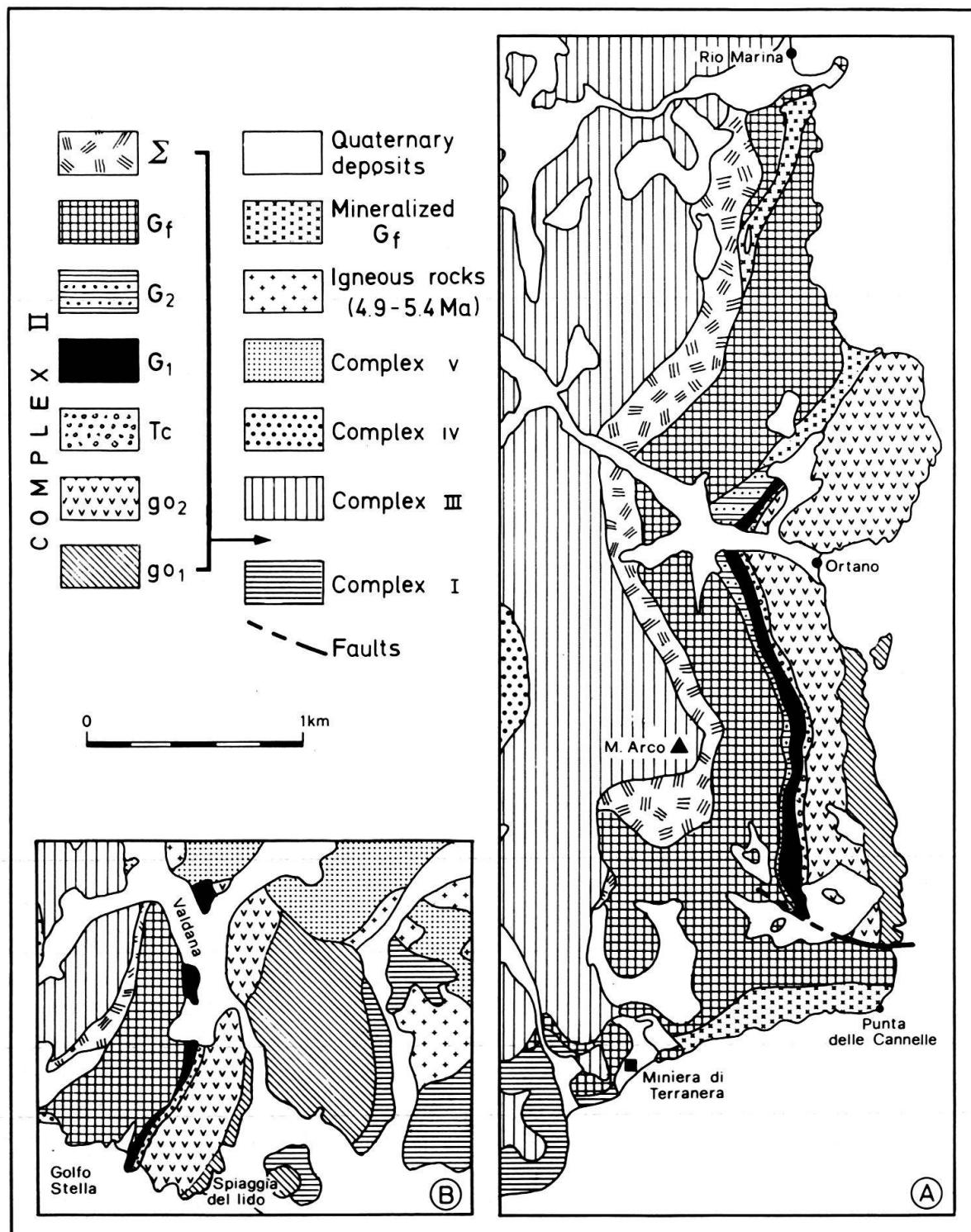
Fig. 2. Geological map of the Ortano-Rio Marina (A) and Spiaggia del Lido-Valdana (B) areas partly modified after BARBERI et al. (1967a):  $\Sigma$ : Serpentinite; G<sub>f</sub>: Phyllite with local Calcschist intercalations; G<sub>2</sub>: Calcschist; G<sub>1</sub>: Ortano marble; T<sub>c</sub>: Vacuolar limestone; go<sub>2</sub>: "Porfiroidi" and "Scisti Porfirici"; go<sub>1</sub>: Spotted Schist.
