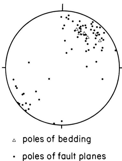
Fig. 6. Distribution of bedding and fault planes in the Monteolimpino tunnel. Lower hemisphere, equal-area stereographic projection.
