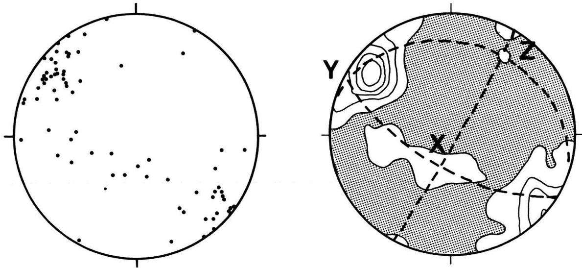
Fig. 7. Directions of strain axes determined with ARTHAUD'S (1969) method. Lower hemisphere, equal-area stereographic projection, contoured at 1.0, 3.0, 5.0, 7.0, 9.0, 11.0, 13.0, times uniform (number of points per 1.35% area).
