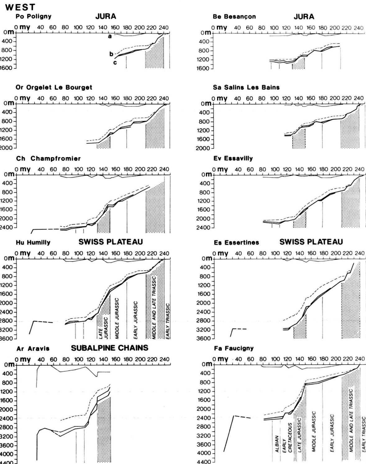
Fig. 3. Geohistory diagrams of the base of the Mesozoic sediments for some characteristic sections of the Helvetic realm, the Swiss Plateau and the Jura (position of the sections: see Fig. 1 and 4).
