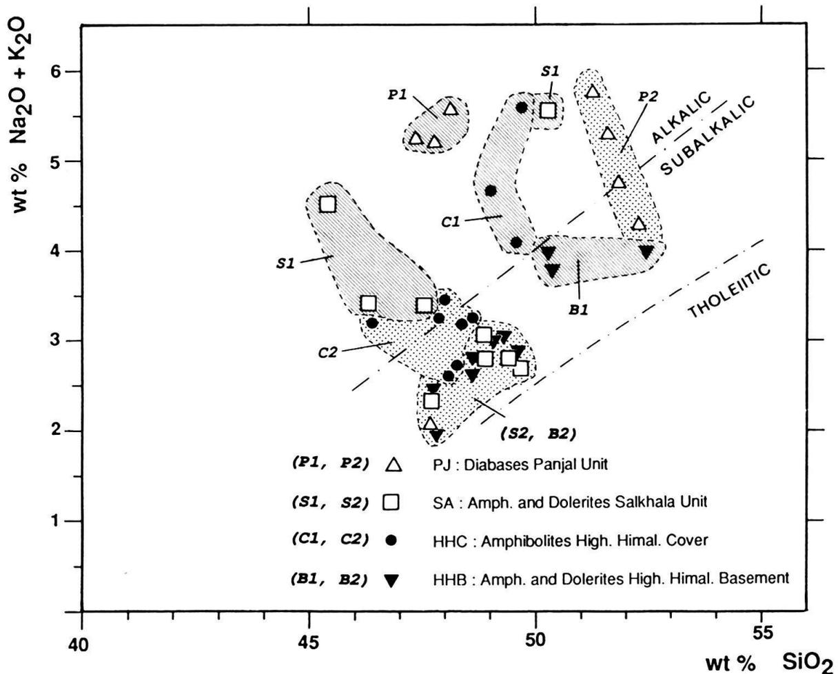
Fig. 6. (Na<sub>2</sub>O+K<sub>2</sub>O) vs. SiO<sub>2</sub> variation diagram. Alkalic-subalkalic boundary after MACDONALD & KATSURA (1964), tholeiitic boundary after KUNO (1968). Analyses are plotted anhydrous and calcite free. Data grouped after tectonic units from the Western Syntaxis area: PJ: Panjal Unit; SA: Salkhala Unit; HHC: Higher-Himalayan cover; HHB: Higher-Himalayan basement.
