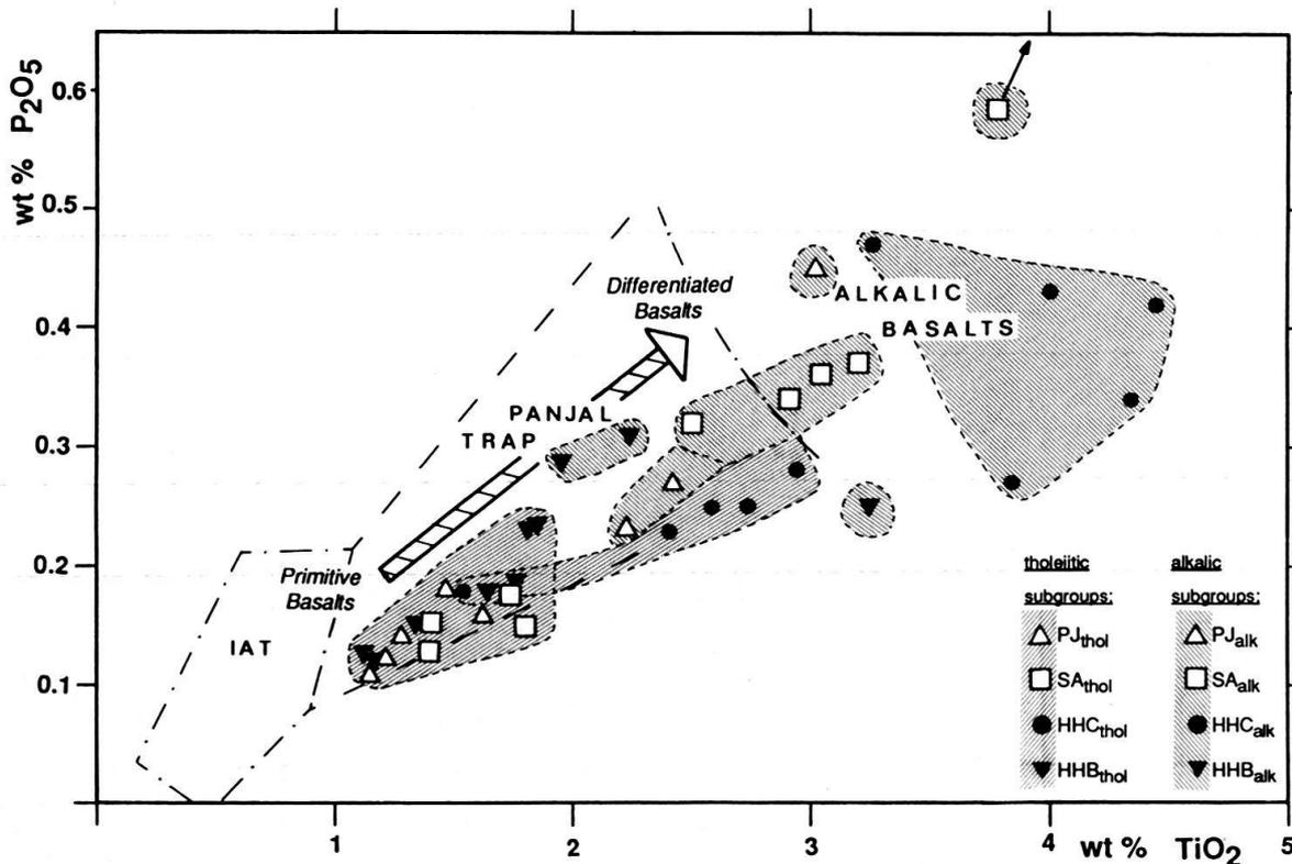
Fig. 7.  $\text{P}_2\text{O}_5$  vs.  $\text{TiO}_2$  variation diagram. Island Arc Tholeiite (IAT) discrimination field and alkalic basalt field from HAWKINS (1980); Panjal Trap distribution field from HONEGGER et al. (1982). Data grouped after tectonic units from the Western Syntaxis area: PJ: Panjal Unit; SA: Salkhala Unit; HHC: Higher-Himalayan cover; HHB: Higher-Himalayan basement.
