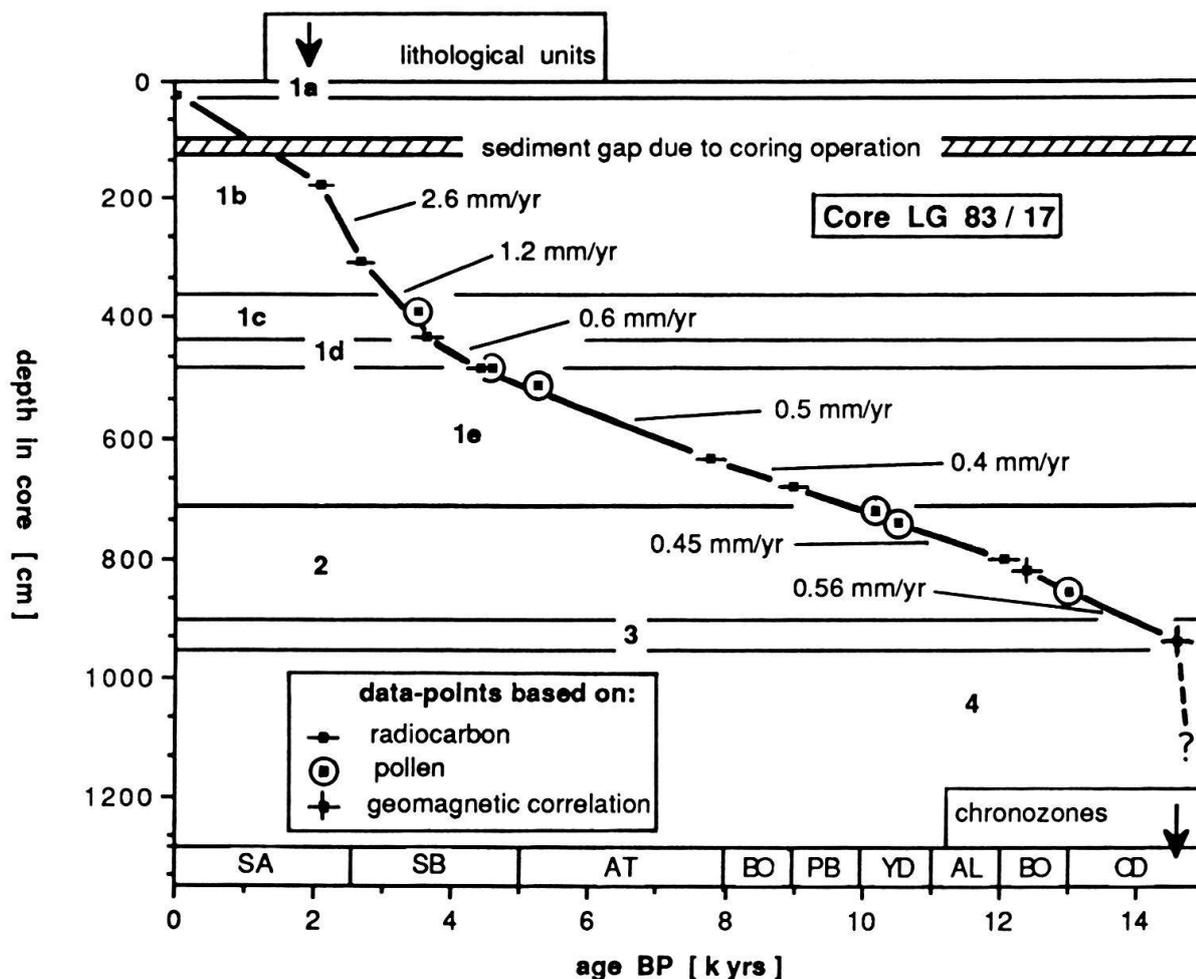
Fig. 2: Radiocarbon, pollen, and geomagnetic ages plotted versus sediment depth. The results of  $^{14}\text{C}$ -measurements are listed in Table 1. The pollen results are discussed by Wick (1989), and the paleomagnetic data points are obtained from Figure 3. (Chronozones after MANGERUD et al. 1974).
