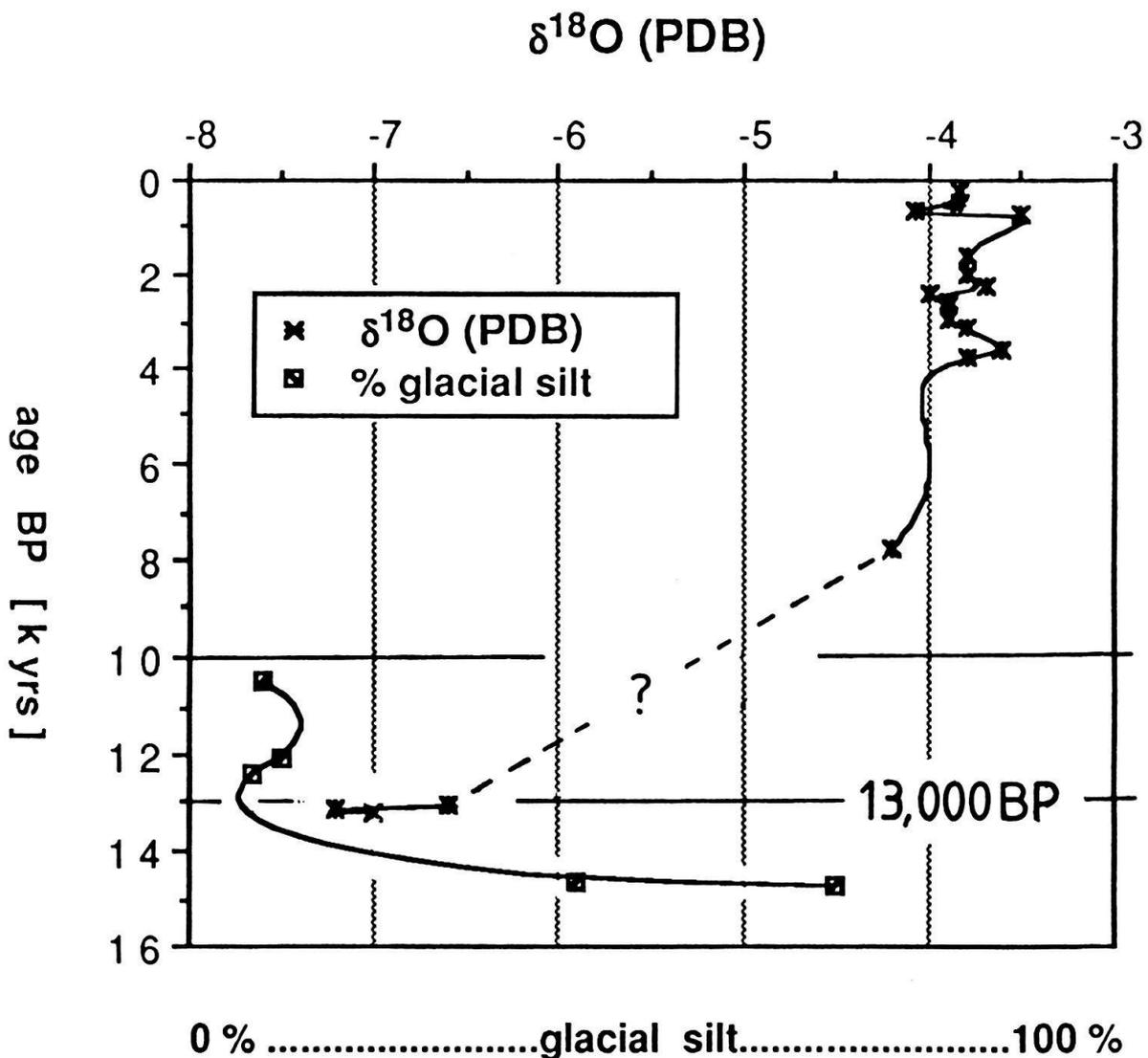
Fig. 6: Oxygen isotope results from benthic deep water ostracods (cores LG 83-7 and LG 83-17) plotted versus time (details are listed in Table 3). The isotope stratigraphy is compared to the amount of glacial silt in bulk samples which was estimated from calcite and dolomite contents. Note that the two gradients of glacial silt and  $\delta^{18}\text{O}$  are displaced by at least 900 years.
