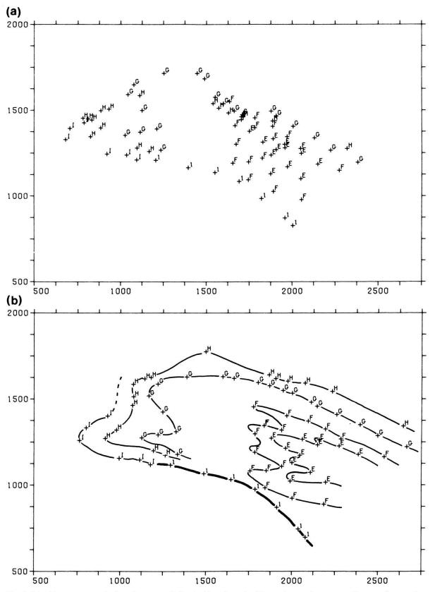
Fig. 3. Machine-contructed plots for part of the Ardève domain. The units are in metres. Crosses denote the positions of projected points on the topographic traces of stratigraphic horizons. Letters identify the stratigraphic horizons of these traces (Tab. 1); numbers denote major faults. (a) Projection direction oblique to the fold axis. (b)
