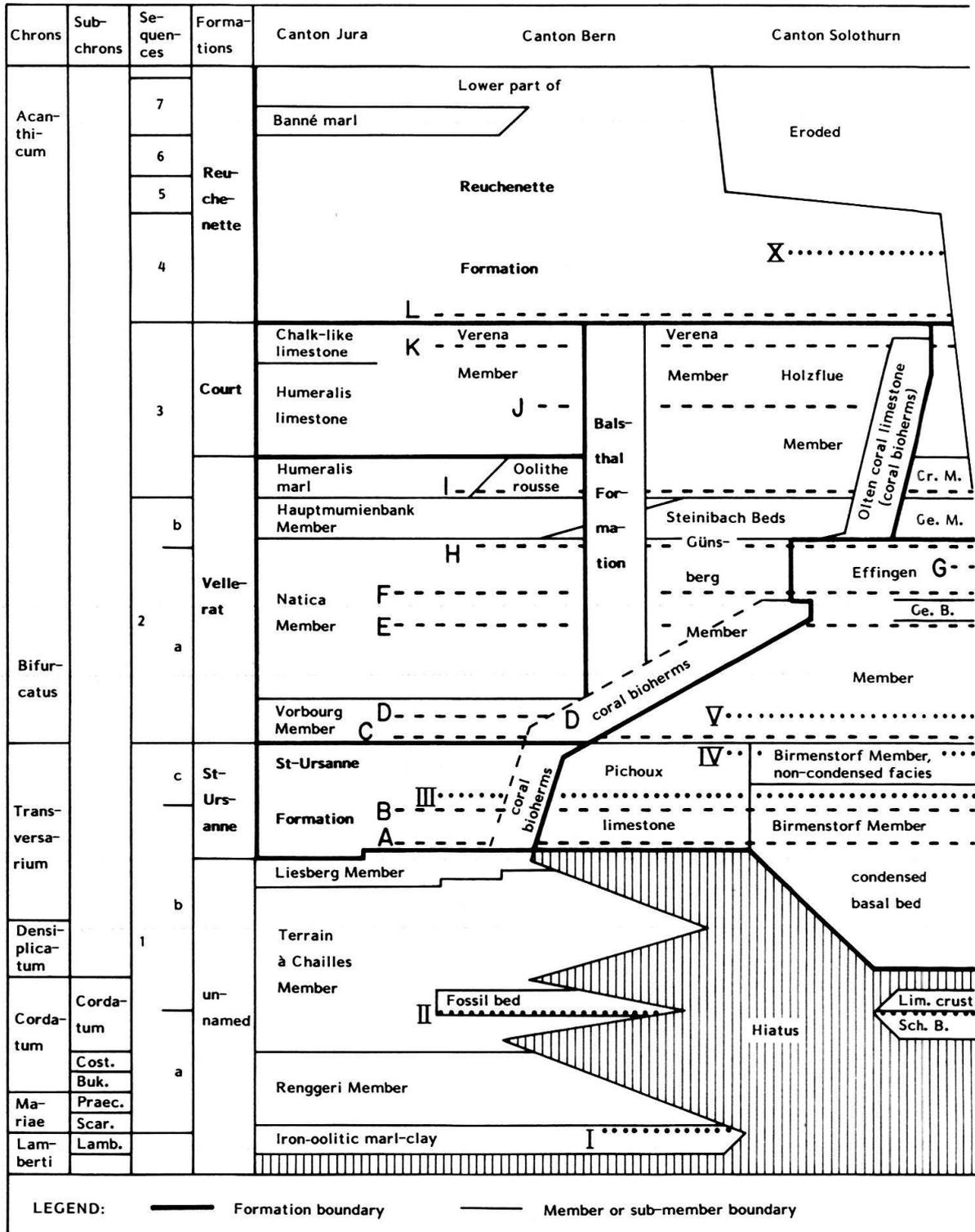
graphic correlations are the effect of low sedimentation rates. The vertical extent of the lithostratigraphic and biostratigraphic units in this table is unrelated to the time represented by the units. Bold lines are formation boundaries.
