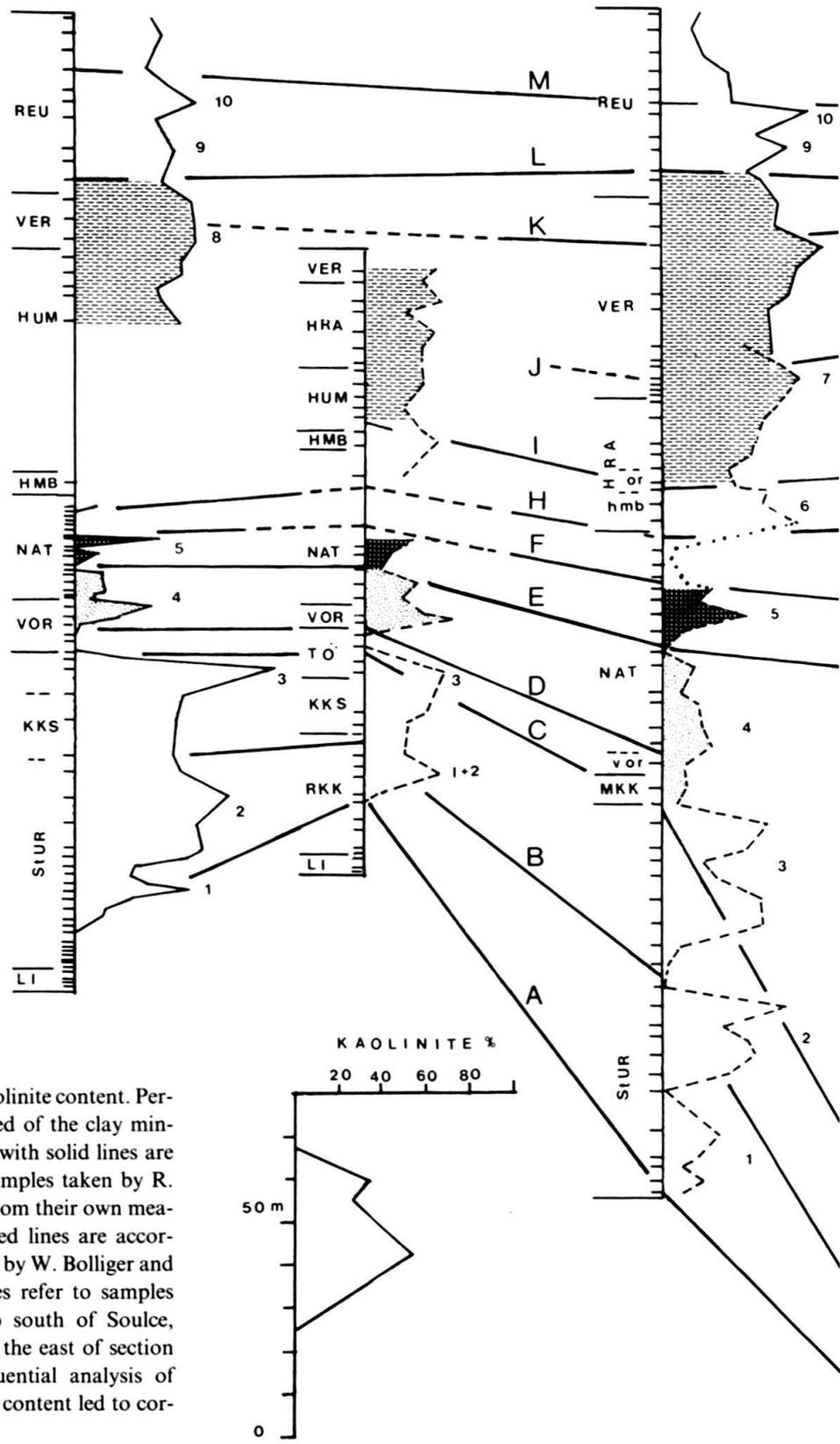
Fig. 10. Profiles of kaolinite content. Percentages are calculated of the clay minerals. Profiles drawn with solid lines are based on analyzed samples taken by R. Gygi and F. Persoz from their own measured sections. Dashed lines are according to samples taken by W. Bolliger and P. Burri. Dotted lines refer to samples taken at an outcrop south of Soulce, several kilometers to the east of section no 6, Pichoux. Sequential analysis of variation in kaolinite content led to correlations A to M.
