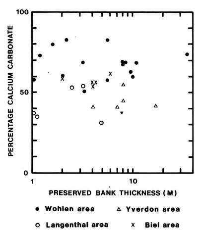
Fig. 7. Plot of calcium carbonate content versus preserved Muschelsandstein bank thickness. Note that banks of high steepness, principally in the Wohlen area, possess high CaCO<sub>3</sub> contents from the large shell fraction. Banks of low steepness, in the Langenthal area have low CaCO<sub>3</sub> contents.
