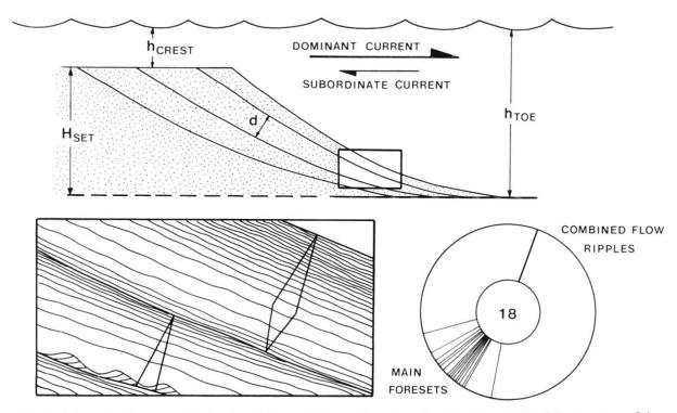
Fig. 11. Schematic diagram of the bank at Mägenwil Naturschutz (locality 19) with a detail of the structure of the cyclically-arranged toesets.
