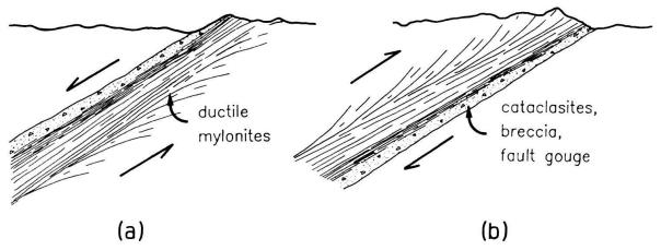
Fig. 11. Asymmetric profiles predicted from Figure 10 for major fault zones with a) normal or b) reverse sense of displacement.
