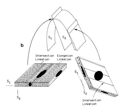
Fig. 4. The relationship between fabric style and position within a fold in an earlier foliation. a) the earlier tectonic foliation,  $S_1$ , and its associated finite strain prior to folding. b) the folded foliation,  $S_1$ , with a newly developed axial plane foliation,  $S_2$ . The resultant tectonic has a linear fabric in the hinge region and a more planar fabric on the limbs.
