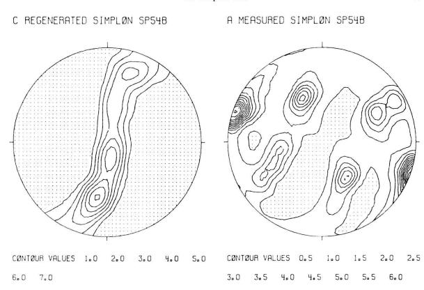
Fig. 9. Contoured upper hemisphere equal area stereoplots of the < a > and c-axis orientation distribution for specimen SP54B (loc. Simplon Dorf, coord. 647.700/116.300). Orientation of the stereoplots is the same as in Plate 2. The < a > pattern was measured directly with a texture goniometer, the c pattern regenerated from the ODF, based on measurements of 9 crystallographic planes, following the method of CASEY (1981).
