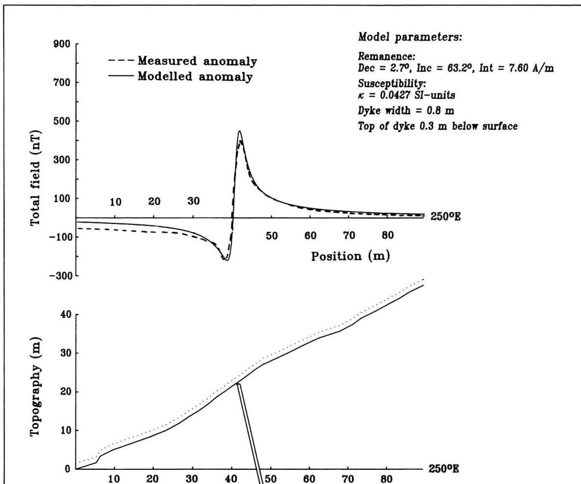
Fig. 6. Comparison between measured (dashed line) and modelled total field anomaly of the dyke on a slope profile at Ramsen.
