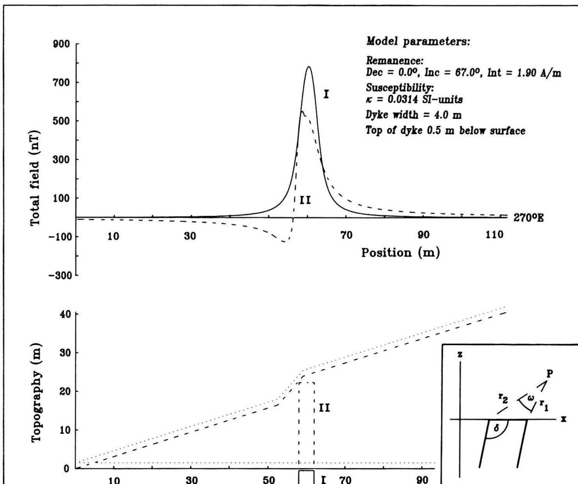
Fig. 5. Effect of topographic step on the total field anomaly of a N-S striking dyke. Dashed lines (Model II) illustrate the situation of an inclined terrain surface with a topographic step, solid lines (I) refer to flat terrain surface. Dotted lines indicate height of the actual measuring profile 1.5 m above terrain surface. The specific model parameters are denoted in the top right corner of the figure. The inset illustrates some parameters used in formulas 1-3.
