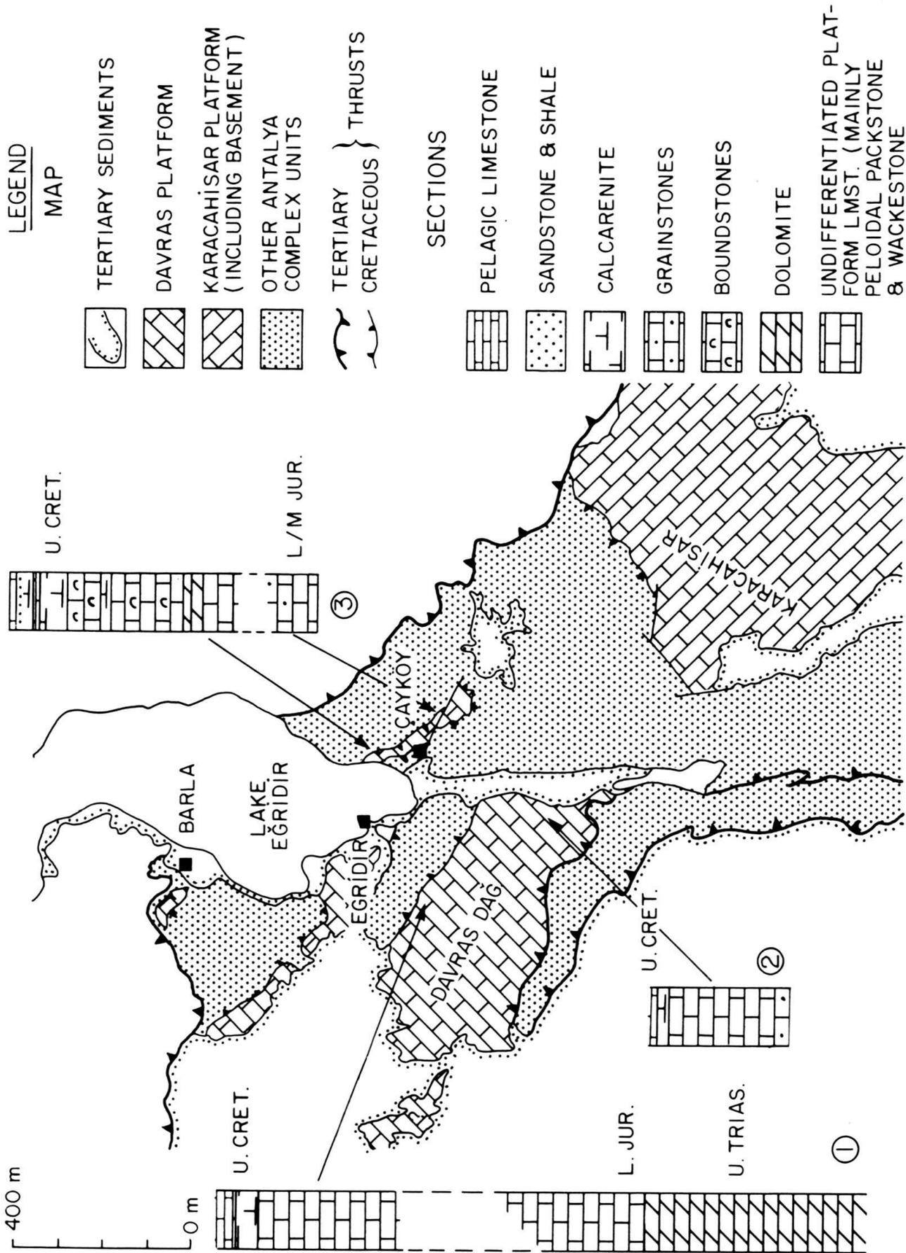
Fig. 7. Davras platform; map and stratigraphic sections. Section 1 is constructed from map and descriptions of GUTNIC et al. (1979). Section 2 after AKBULUT (1977). Section 3 measured by the author. Map compiled from GUTNIC et al. (1979), DUMONT (1976) and the author's field maps. Location of Lake Eğirdir is shown in Figure 2.
