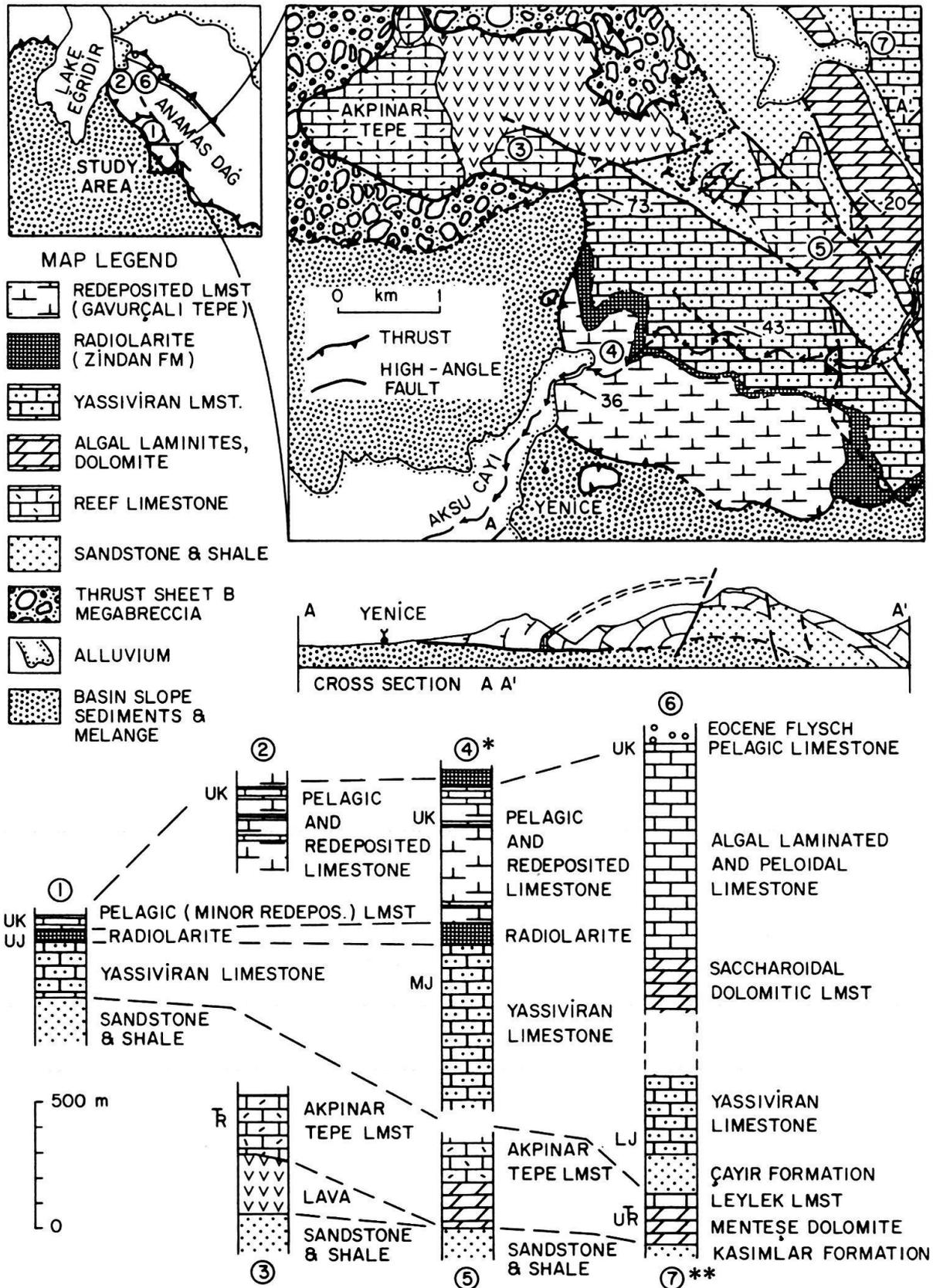
Fig. 4. Margin of the Anamas-Akseki platform in the area east of Lake Eğirdir (located in Figure 2). Top: Map and cross section of thrust sheet A (map shows structure and location of stratigraphic sections). Bottom: Stratigraphic sections. \*Section 4 in part after DUMONT et al. (1980). \*\*Section 7: thicknesses after GUTNIC (1977).
