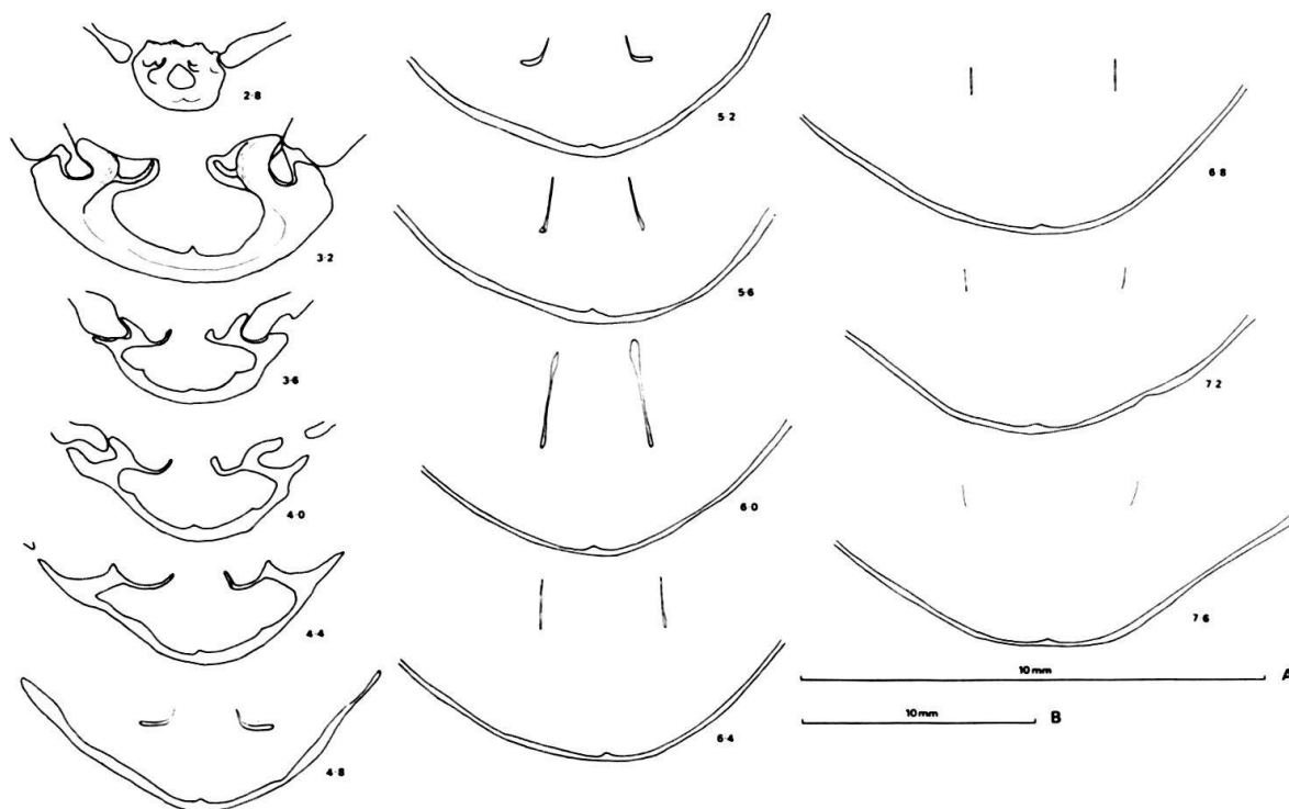
Fig. 10. Serial sections through Loriolithyris russillensis latifrons (Pictet). The initial concave shape of the hinge plates is shown at 2.8 and 3.2, the first clear indication of attached crural bases occurring at 4.4. Transverse band not preserved. Section 3.2 is enlarged in order to show detail of the juvenile hinge plates. 608/3/1, Neuchâtel Coll., Upper Valanginian, Villers-le-Lac, Doubs. Dimensions of specimen: L. 21.25, W. 20.25, T. 13.25. A = scale for section 3.2. B = scale for the remaining sections.
