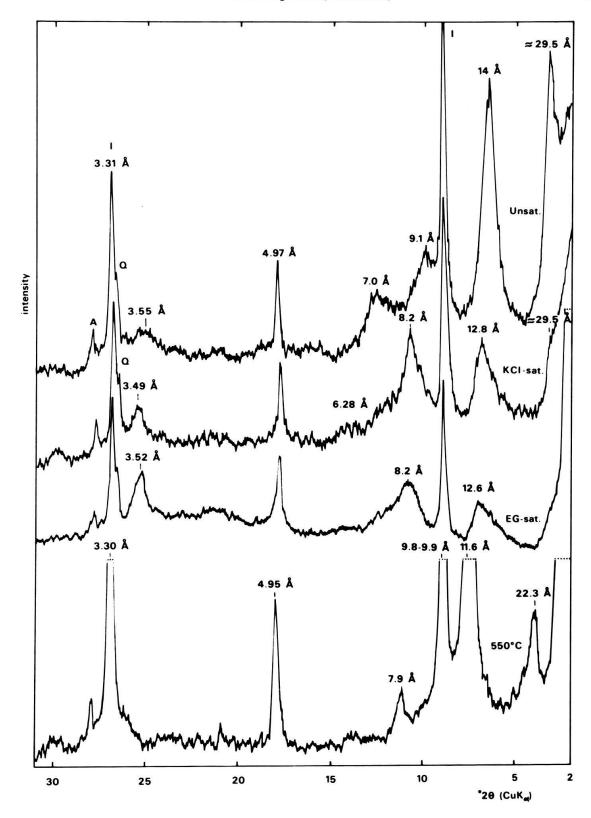
Fig. 4. X-ray diffraction traces of unsaturated, KCl-saturated, ethylene-glycol (EG) saturated (during 48 hours), and 550 °C heated (2 hours) oriented – 2 μm fractions of sample containing partly ordered mica-chlorite and chlorite-vermiculite mixed-layers. Sample No.119A from the "mylonitized zone" on the western margin of the Olympos window, south of Kokkinoplos (Stalamata section of GODFRIAUX in DERCOURT et al. 1977, p. 49). I = illite or muscovite; Q = quartz; A = albite or plagioclase.
