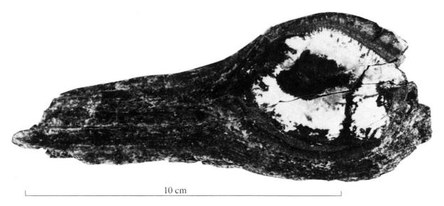
Fig. 9. Manganese nodule (PVB 1663). The black core consists of garnet and spessartite, the surrounding light coloured shell is composed of spessartite and quartz. The nodule is embedde in a fine laminated schist with alternating quartz-rich bands and spessartite and (or) mica-rich bands. Notice the manganese dendrites along the boundary of the light shell.
