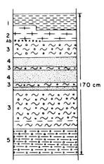
Fig. 2. Detail from the section through the Combin zone (along the path Zermatt-Trift, altitude 1970 m). 1= Calcschists, 2= marbles, 3= albite-rich micaschist, 4= muscovite quartzite with intercalations of 3, 5= chlorite-phengite-albite gneiss.
