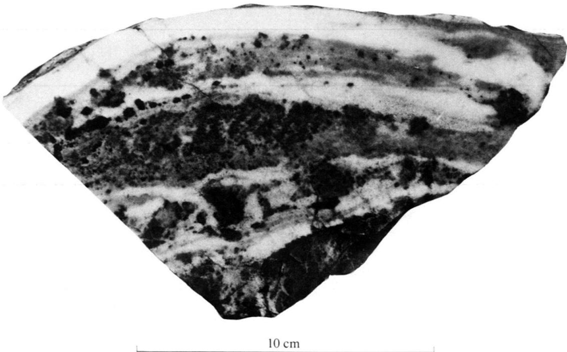
Fig. 11. Sample (PVB 1660a). White quartz-rich bands alternate with bands containing the assemblage quartz + spessartite (grey and dark grey). The black spots (upper right) represent limonitic relicts of a weathered carbonate mineral.
