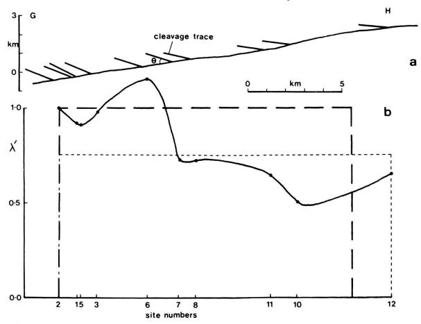
Fig. 6. Calculation of the bulk extension along section line *GH* (Fig. 1), using the method of Hossack (1978). Diagram *a* shows the trace of the Glarus Thrust, constructed using data given by Trümpy (1969) and SCHMID (1975), the oblique lines are the orientations of strain ellipse long axes projected onto the section plane.
