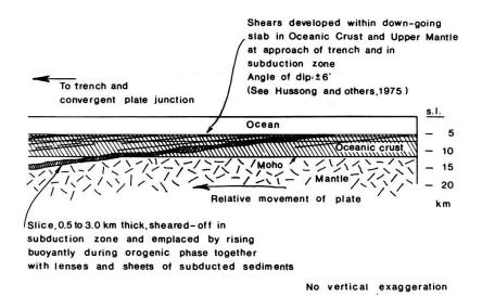
Fig. 2. Suggested mechanism for origin of ophiolite slices.
