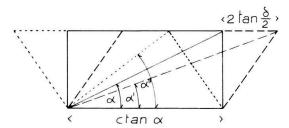
Fig. 1. Deformation of a thrust plane by a single kink band in locking position (simple shear). a = original dip of thrust, a'(a'') = angle with respect to bedding after positive (negative) shear,  $2 \tan \delta/2$  ( $-2 \tan \delta/2$ ), where  $\delta = \text{dip of the kinked beds (originally horizontal)}$ .
