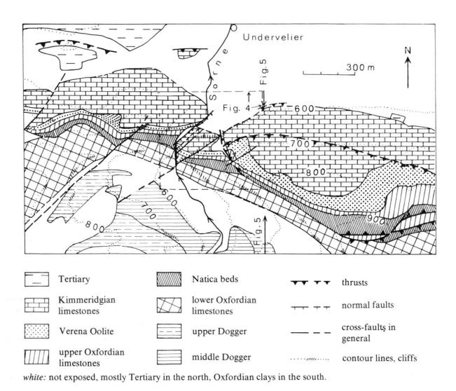
Fig. 3. Fault contacts in the north limb of the Raimeux anticline south of Undervelier, 40 km SW of Basel, simplified map. Interpretation of fault contacts on the east side of the Sorne river gorge as a graben (compare Fig. 4).
