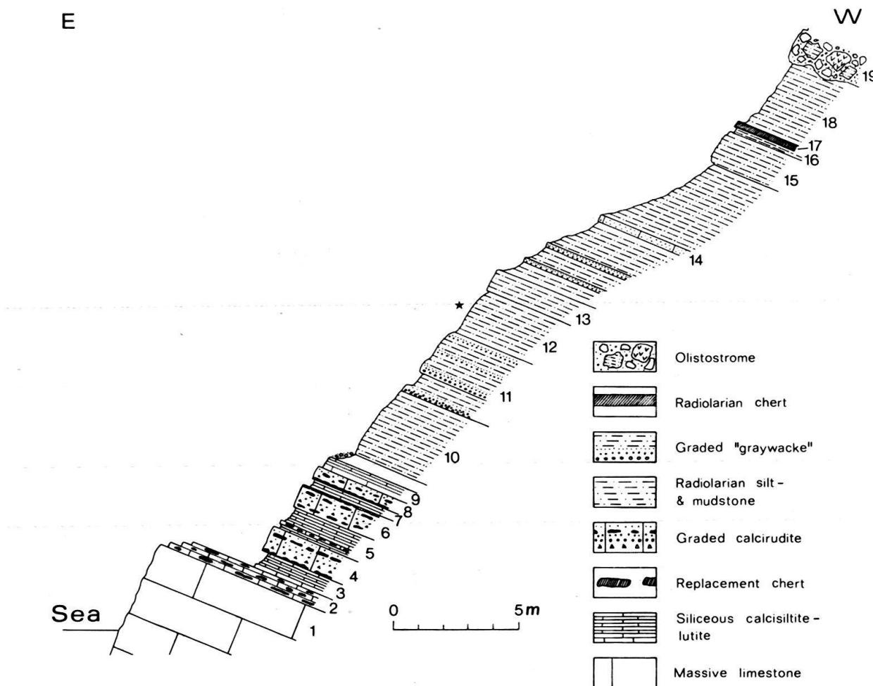
Fig. 2. Stratigraphic section in the top of the Cladocoropsis Limestone and the base of the Diabase-Chert Formation, beach of Achladi, Evvoia. Description in the text. \*Radiolarian fauna.
