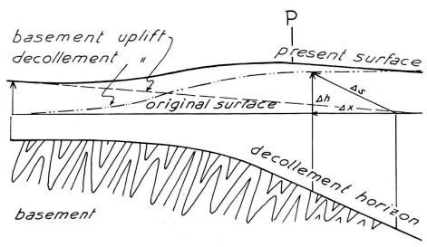
Fig. 2. Superposition of decollement induced uplift and true basement uplift which transcends the boundary of decollement.
