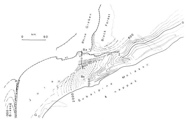
Fig. 3. Present position (in meters) of the top of marine Miocene = total uplift since deposition which was close to sea level. Solid contours after Lemcke (1974). Additions (broken contours) are based on data along the northern border of the eastern Jura, on information given by Lefavrais-Raymond (1962) for the Bresse graben, and on interpolation between Lemcke's contours and Essertines-1 (the value for Pfaffnau-1 is too high, that of Courtion-1 too low in this simple interpolation map).
